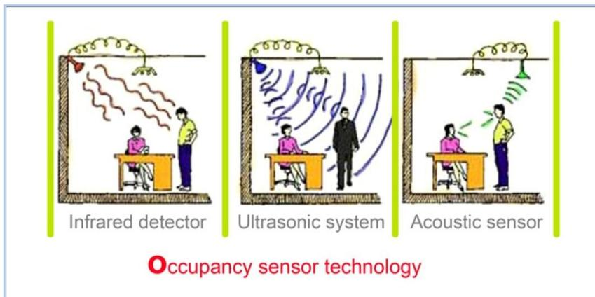
Figure 6: Occupancy sensor technology (www.iklimnet.com)
