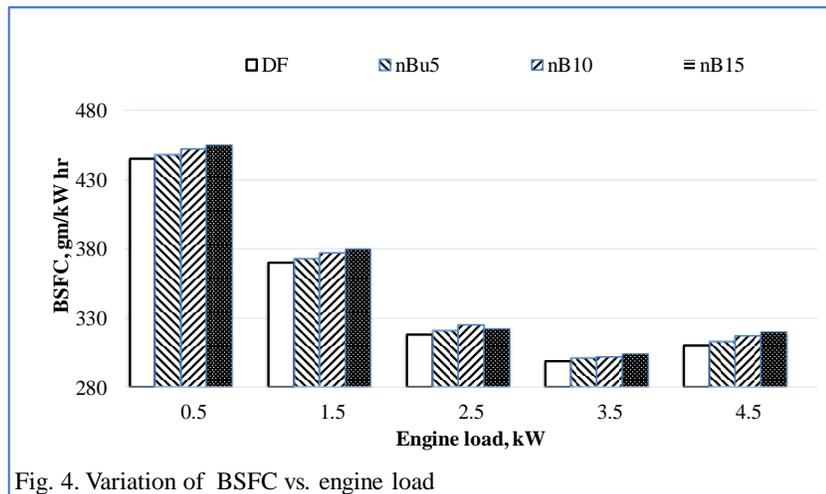
Fig. 4. Variation of BSFC vs. engine load
