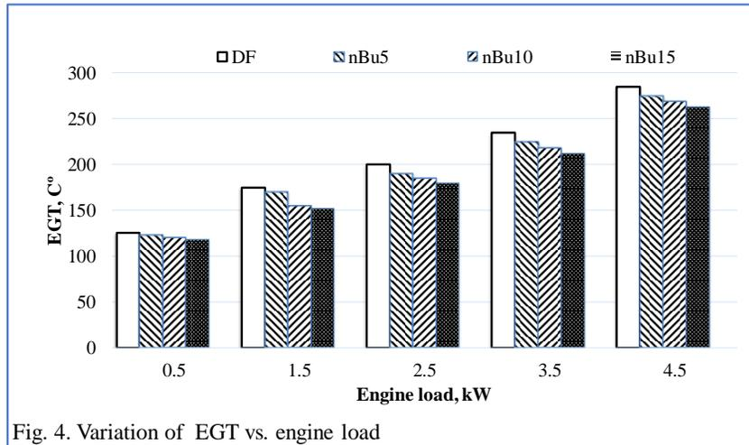
Fig. 4. Variation of EGT vs. engine load
