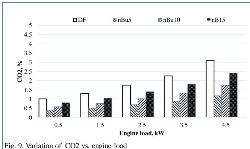
Fig. 9. Variation of CO<sub>2</sub> vs. engine load
