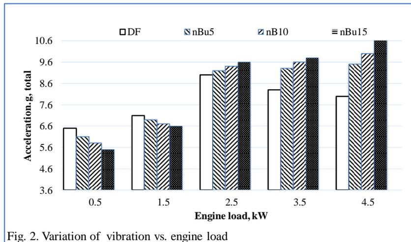
Fig. 2. Variation of vibration vs. engine load
