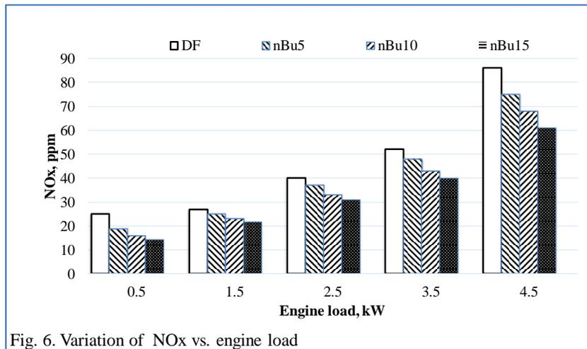
Fig. 6. Variation of NOx vs. engine load
