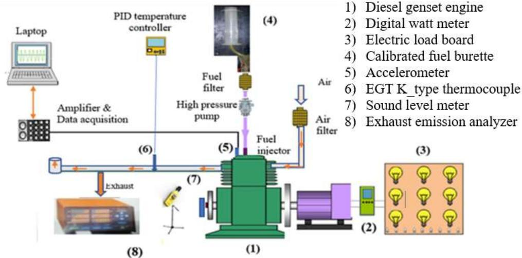
Fig. 1. A schematic diagram of experimental setup.
