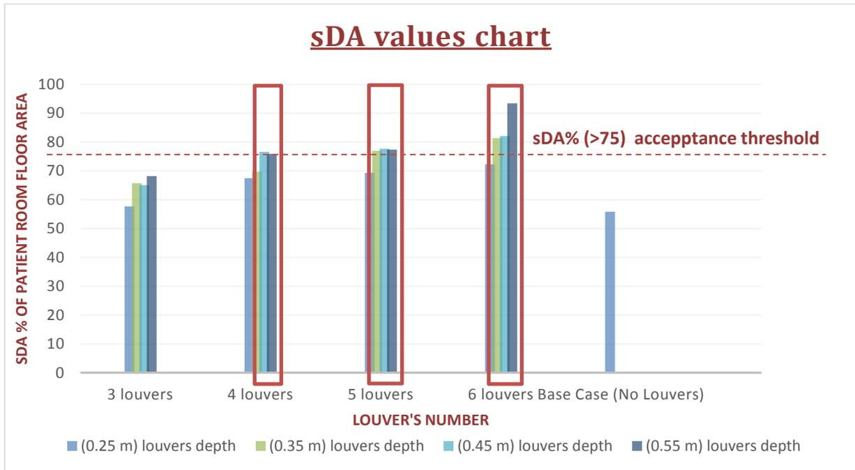
**Fig. (4):** Comparison of sDA results of modeled cases and base case highlighting the successful cases.
