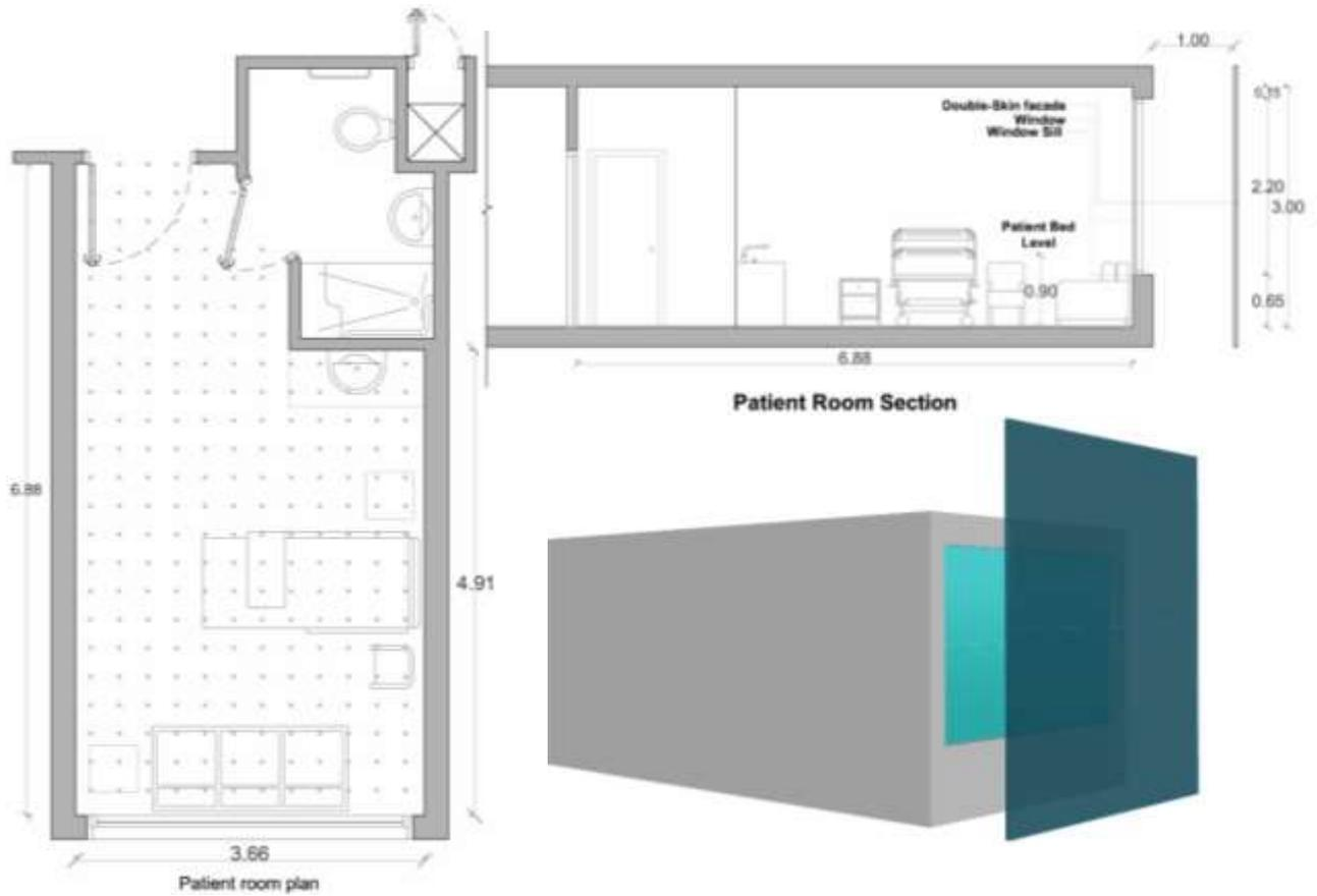
**Fig. (3):** Floor plan, section, and a perspective shot of the tested patient room without DSF daylighting.
