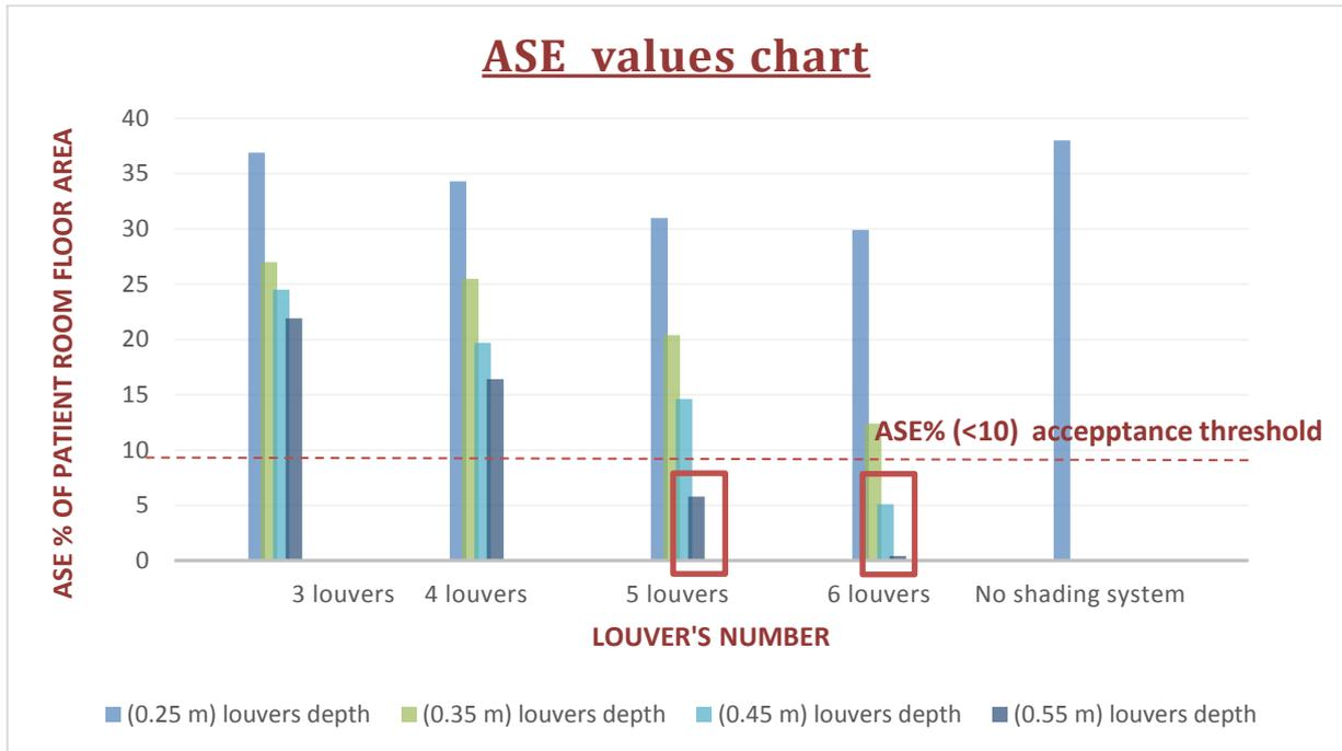
Fig. (5): Comparison of ASE results of modeled cases and base case highlighting the successful cases.
