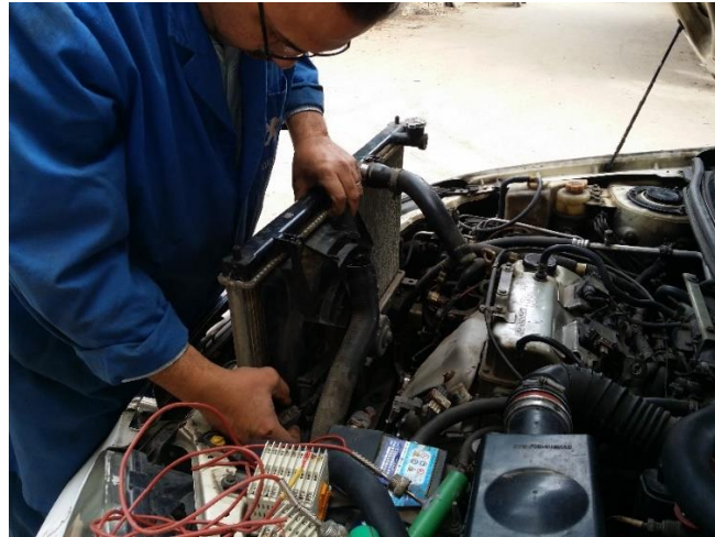
Fig.2: Fixing CR in its original place after mounting thermocouple sensor
