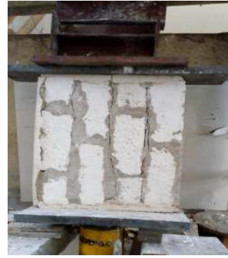
b. Prism constructed using mortar no 4.
