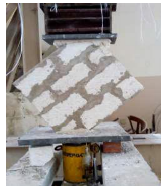
b. Prism constructed using mortar no 4
