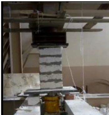
a. Prism constructed using mortar no 1.
