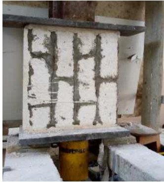
a. Prism constructed using mortar no1.
