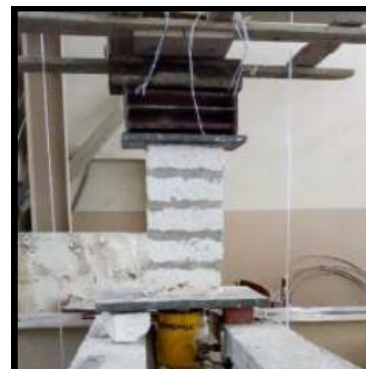
b. Prism constructed using mortar no 4.
