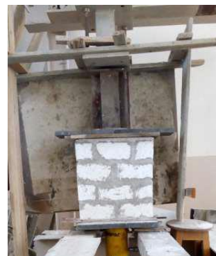
b. Prism constructed using mortar no 4.
