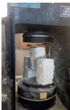
a. Prism constructed using mortar no. (1) b. Prism constructed using mortar no. (4) Figure 13. The failure mode of masonry prisms under shear test
