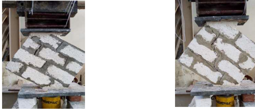
a. Prism constructed using mortar no 1 b. Prism constructed using mortar no 4 Figure 18. Failure mode of prisms under in-plan splitting tensile test with \theta = 45^\circ
