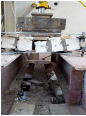
a. Prism constructed using mortar no 1 b. Prism constructed using mortar no 4 Figure 20. Failure mode of prisms - out of plane bending.
