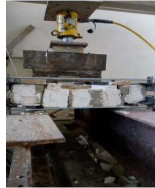
a. Prism constructed using mortar no 1 b. Prism constructed using mortar no 4 Figure 20. Failure mode of prisms - out of plane bending.
