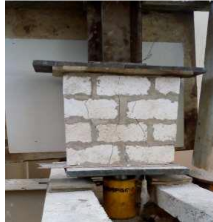
a. Prism constructed using mortar no1. b. Prism constructed using mortar no 4. Figure 14. Failure mode of prisms under in-plan splitting tensile test with \theta = 0^\circ
