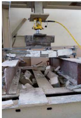
a. Prism constructed using mortar no 1 b. Prism constructed using mortar no 4 Figure 21. Failure mode of out of plane bending-tension parallel to bed joints.
