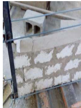
a. Prism constructed using mortar no 1 b. Prism constructed using mortar no 4 Figure 21. Failure mode of out of plane bending-tension parallel to bed joints.
