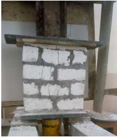
a. Prism constructed using mortar no1. b. Prism constructed using mortar no 4. Figure 14. Failure mode of prisms under in-plan splitting tensile test with \theta = 0^\circ
