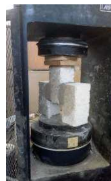
a. Prism constructed using mortar no. (1) b. Prism constructed using mortar no. (4) Figure 13. The failure mode of masonry prisms under shear test
