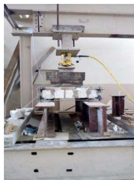
b. Prism constructed using mortar no 4.
