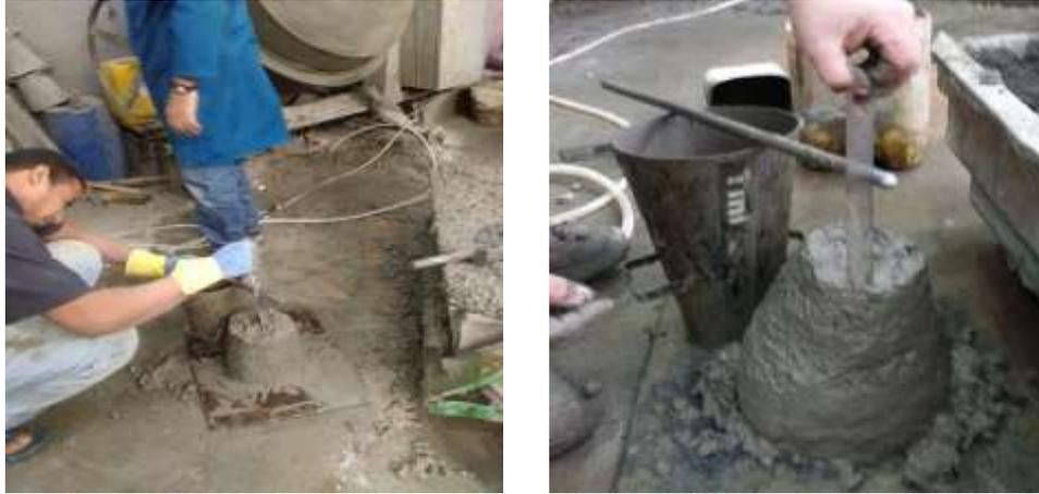
Fig.3: Slump after 30 minutes
