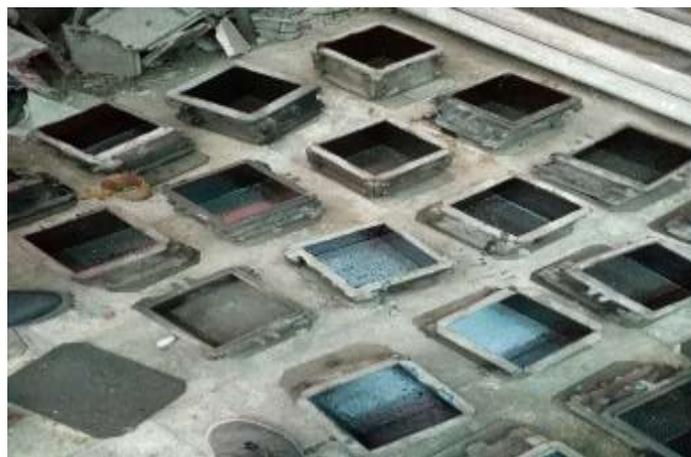
**Fig.2: concrete specimens molds**
