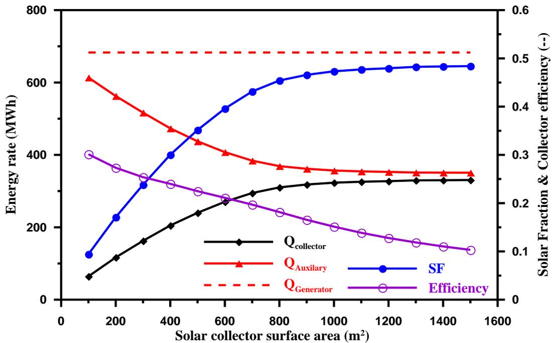
Fig. 11 Effect of solar collector area in energy rate, solar fraction and collector efficiency.
