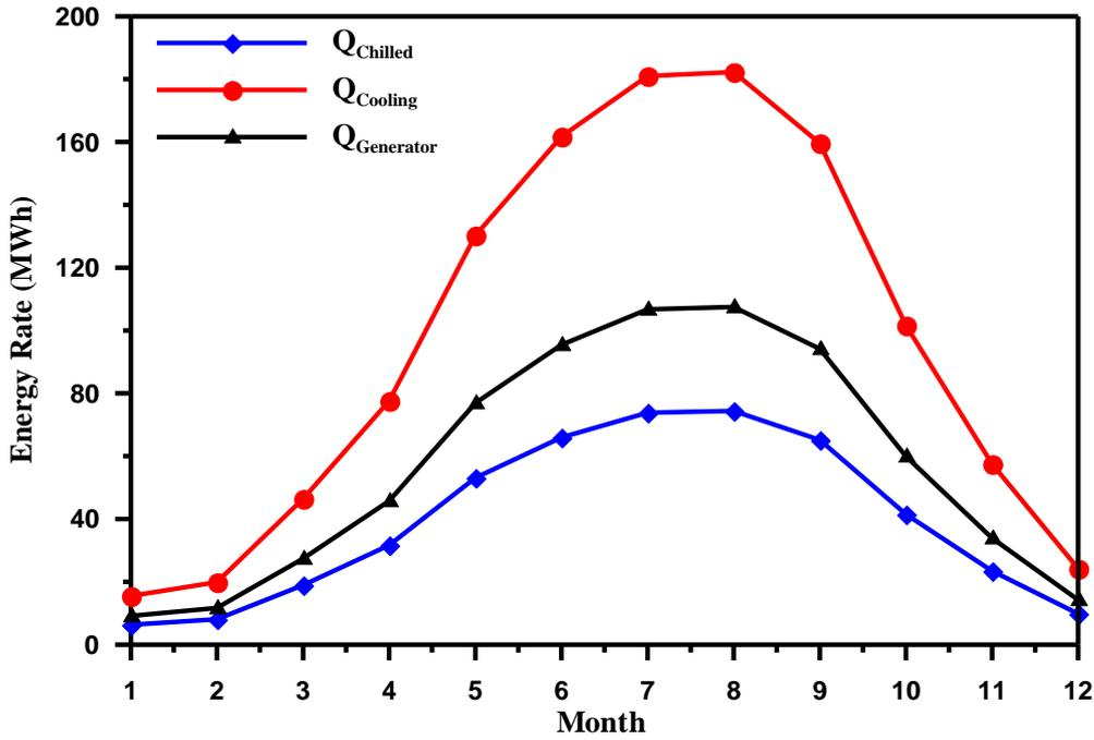
Fig. 14 Monthly chilled, cooling and generator energy rates for proposed solar cooling system.
