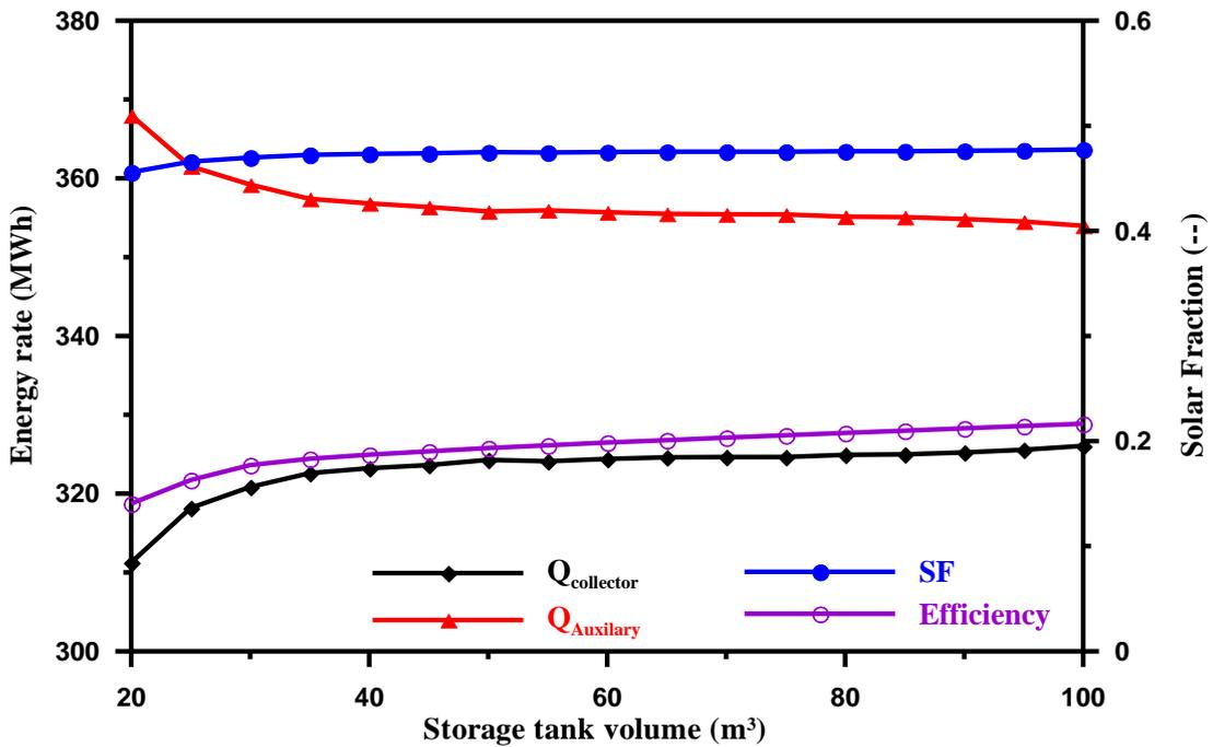
Fig. 13 Energy rate, collector efficiency and solar fraction verses storage tank volume.
