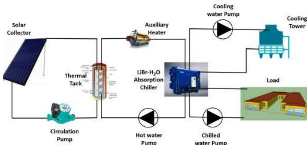
Fig. 1 Schematic diagram of a solar driven air-conditioning system.
