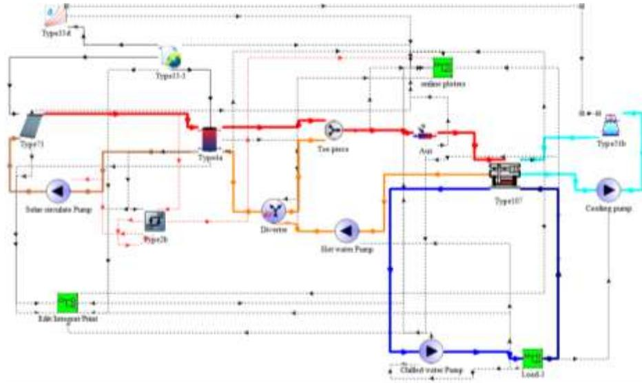
Fig. 4 TRNSYS model of the alternative air-conditioning system.
