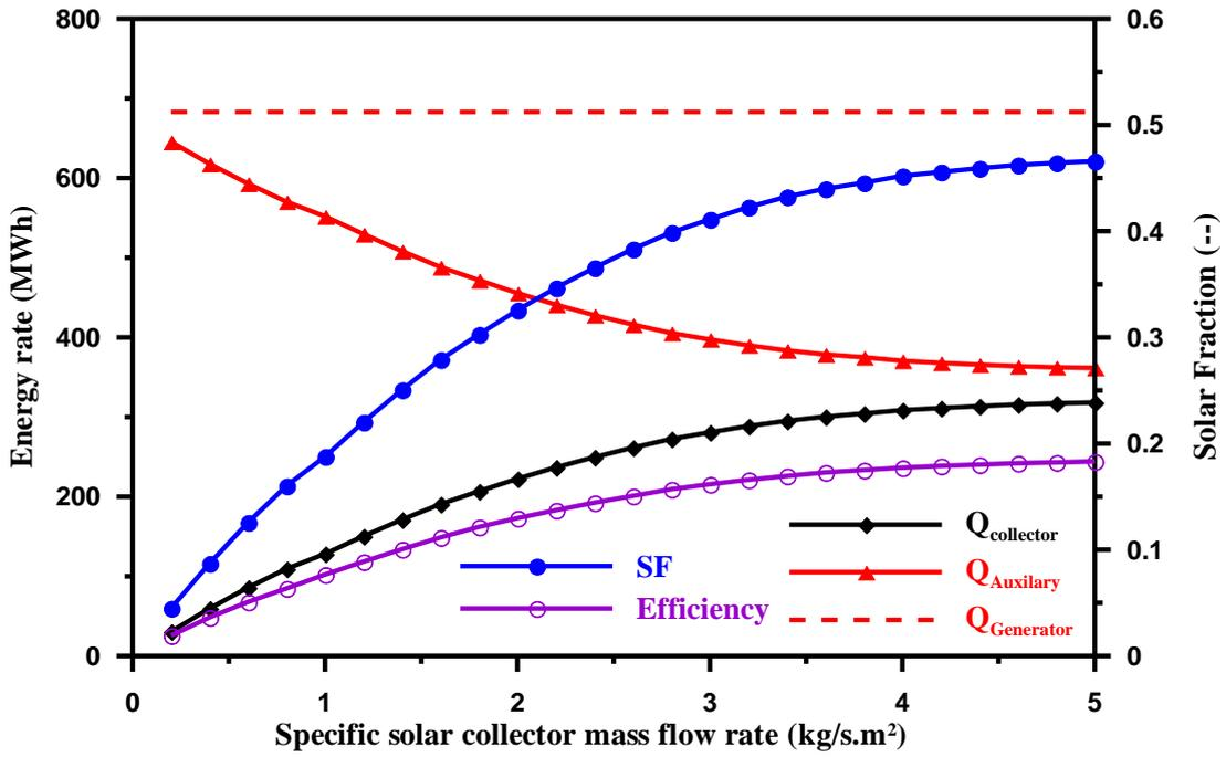
Fig. 12 Variation of energy rate, solar fraction, and collector efficiency with solar collector flow rate.
