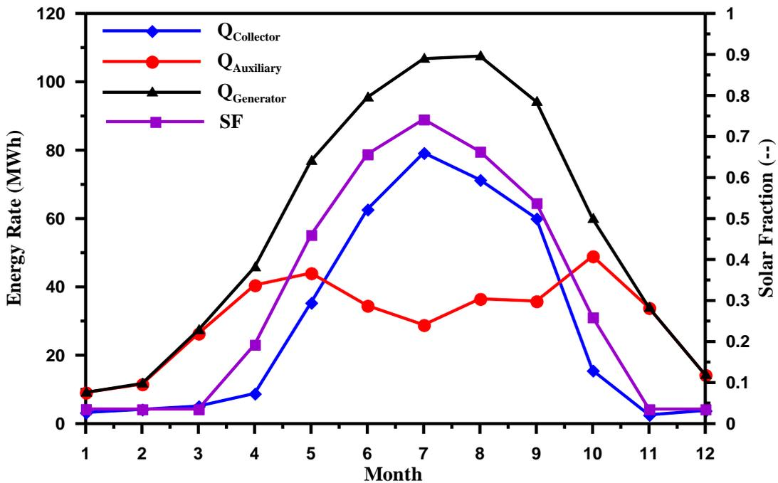
Fig. 15 Monthly chilled, cooling, generator energy rates and solar fraction for proposed solar cooling system.
