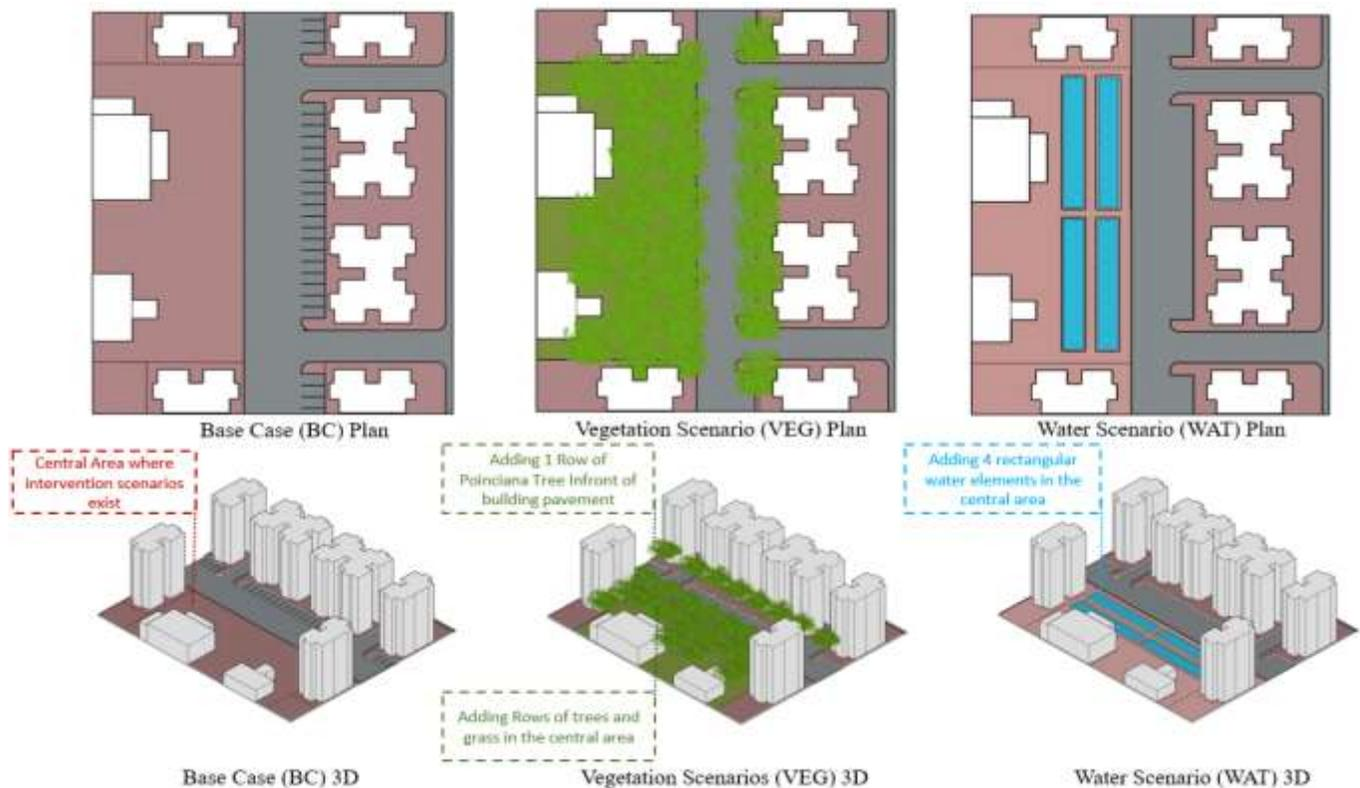
Figure 4 2D plan and 3D showing the base case (BC), Vegetation (VEG) Scenario and Water Scenario, Source: The researcher
