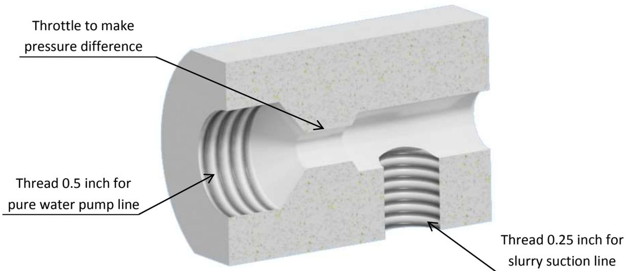
Fig.7 Half section of the Teflon ejector
