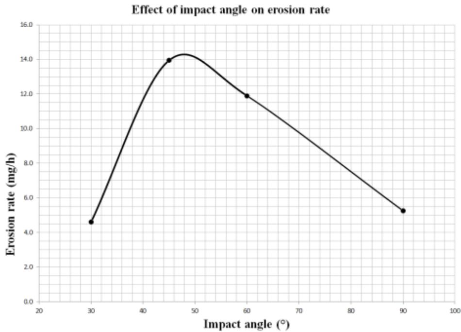
Fig.10 Slurry erosion rate of HDPE for different impact angles, at impact velocity 6 [m/s].
