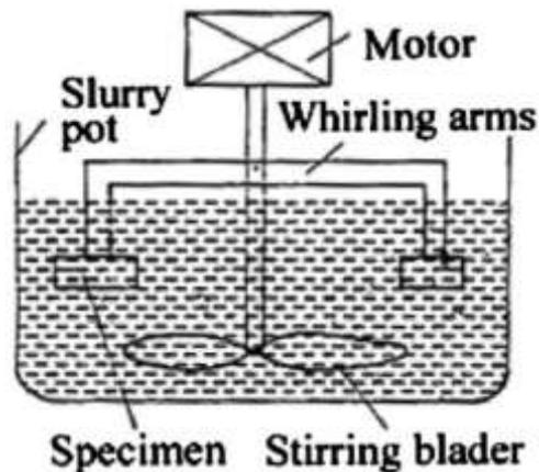
Fig.1 Schematic diagram of slurry pot [3]
