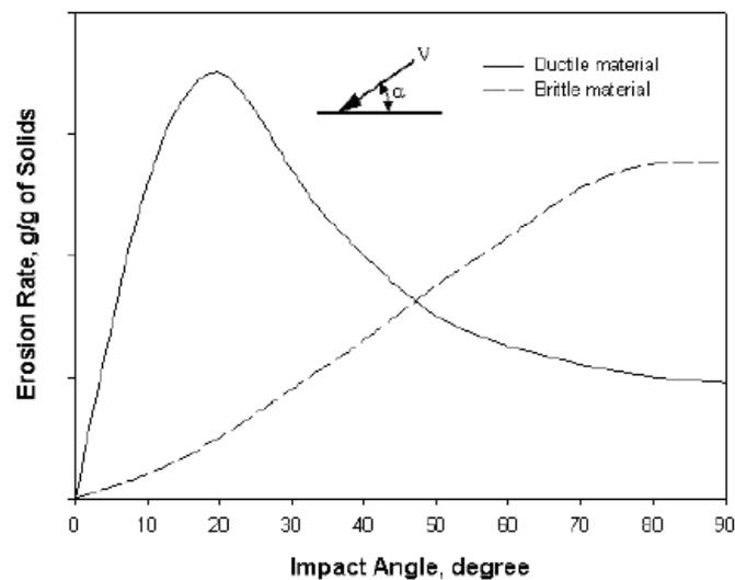
Fig.3 Variation of erosion rate according to impact angle for ductile and brittle materials [4]
