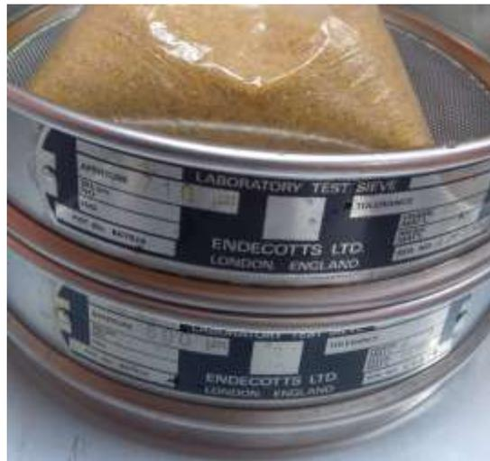
Fig.9 Solid particles, 710  $\mu\text{m}$  and 600  $\mu\text{m}$  sieves
