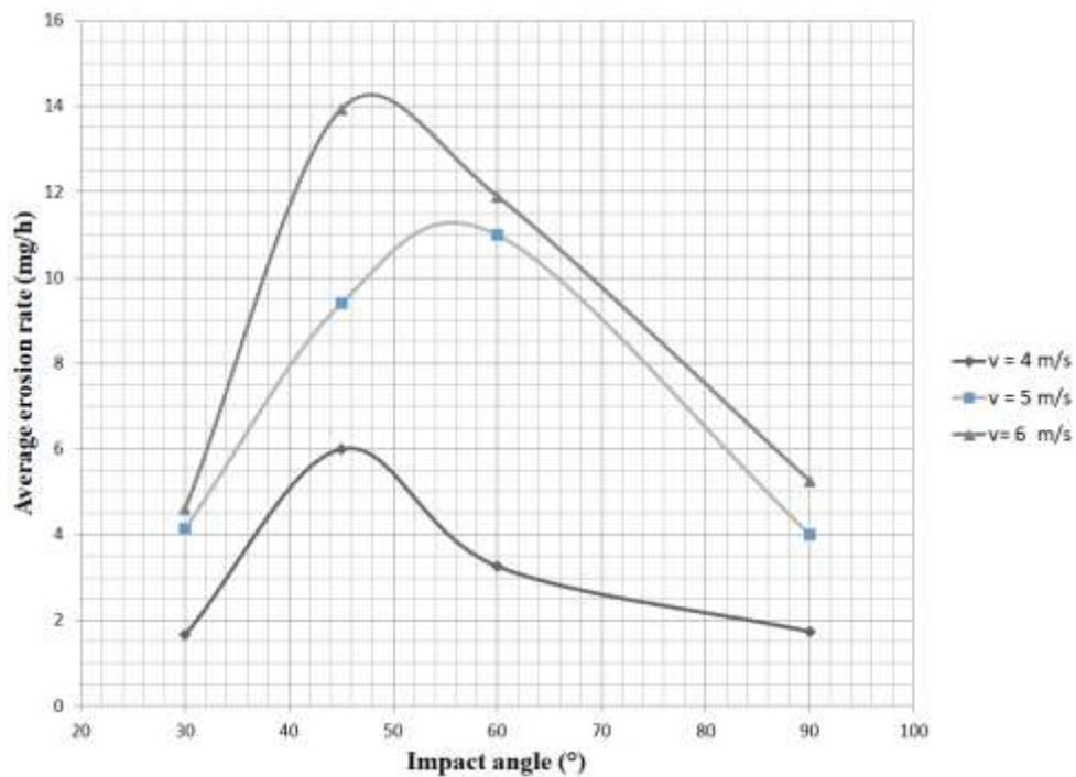
Fig.11 Slurry erosion rate of HDPE for different impact velocity and impact angles
