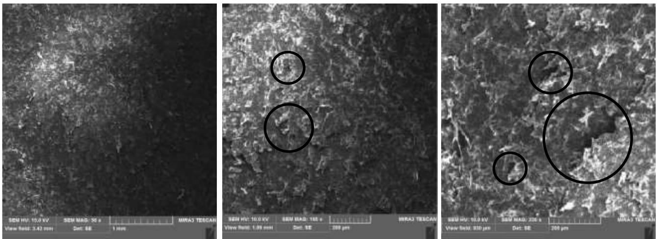
Fig.13 SEM examination image for HDPE sample tested at 90° impact angle and 5 [m/s] impact velocity
