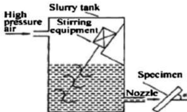
Fig. 2 Schematic diagram of jet impingement tester [3]
