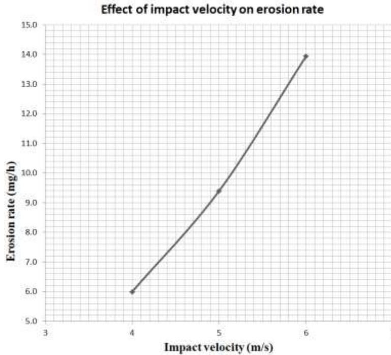
Fig.12 Slurry erosion rate of HDPE for different impact velocity at 45° impact angle
