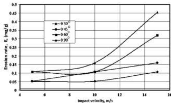
Fig.4 Relation between erosion rate and impact velocity of a polymeric paint-films [3]
