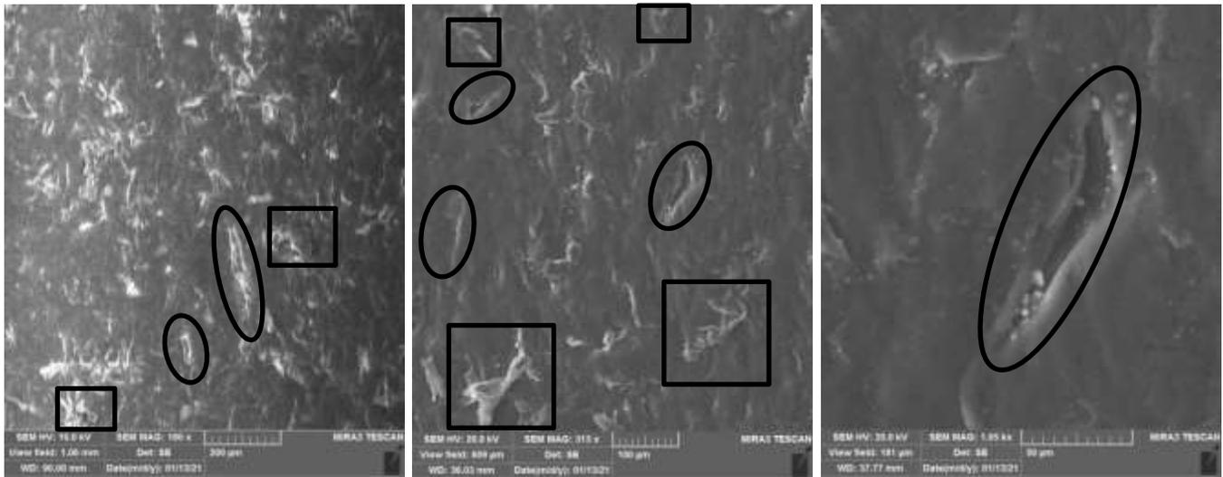
Fig.14 SEM examination image for HDPE sample tested at 30° impact angle and impact velocity 6 [m/s]
