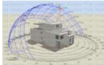
Figure 25 showing the shading areas on the southeast façade and on the roof south shaded area at 2:00 pm on 21st August. (Adapted by researcher with DesignBuilder)
