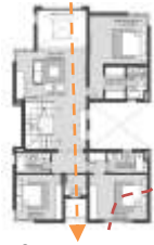
Figure 29 first floor plan with added opening window on the east south facade to enhance cross ventilation and
