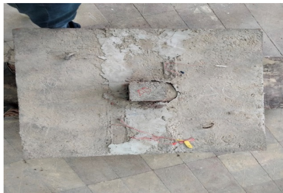
Fig. 13 The crack pattern in the compression side around the columns of specimens A0 and A1.
