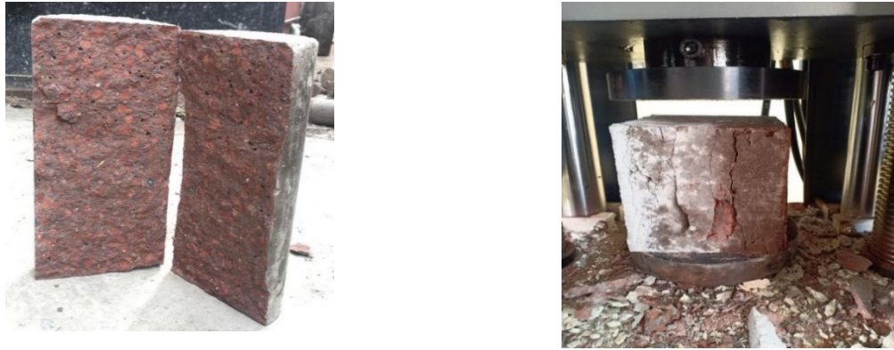
(a) Two halves of a cylinder specimen after tension test.
