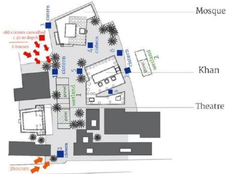
Fig (12): the underground water control system
