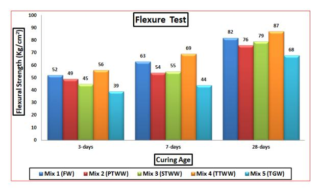
Figure (6): Influence of different types of Treated wastewater on Concrete bending moment at various curing age
