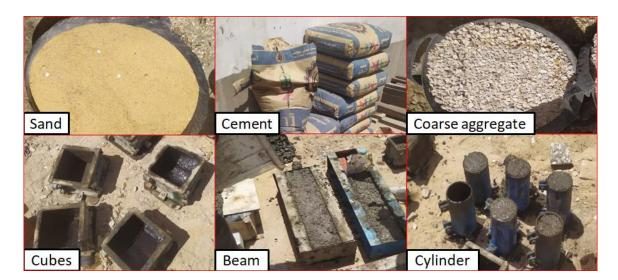
Figure (2): Materials, Samples preparation in laboratory
