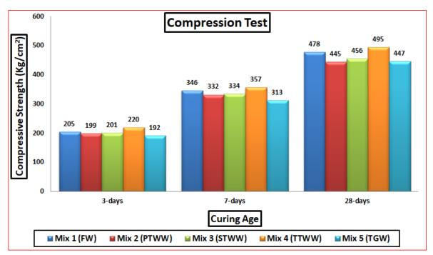
Figure (4): Influence of different types of Treated wastewater on Concrete compressive strength at various curing age
