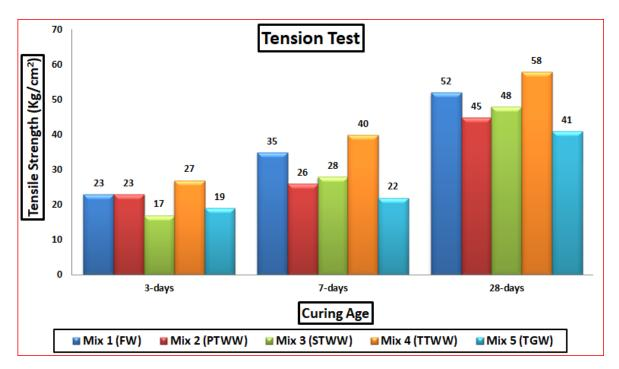
Figure (5): Influence of different types of Treated wastewater on Concrete tensile strength at various curing age
