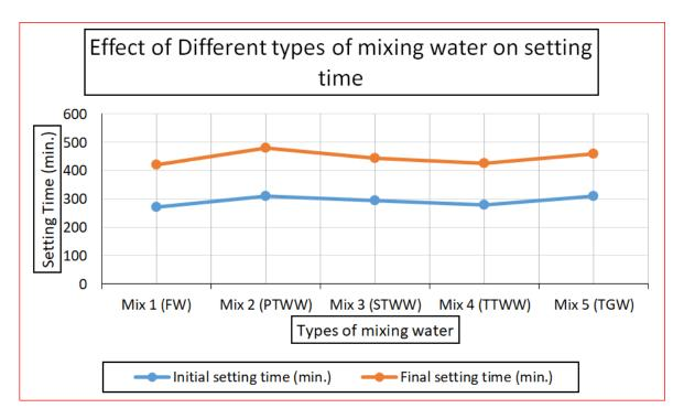
Figure (7): Effect of Different types of mixing water on setting time
