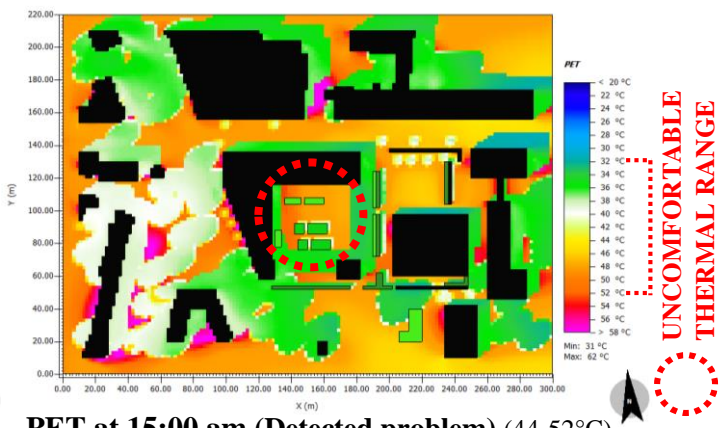
PET at 15:00 am (Detected problem) (44-52°C)
