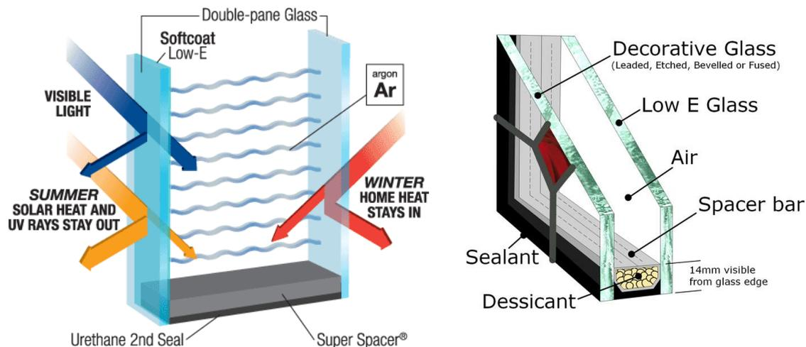
Fig. 12. Double glazed window section (13)
