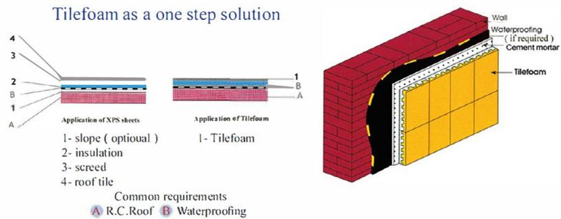
Fig. 13. Tile foam insulation boards layers (13)
