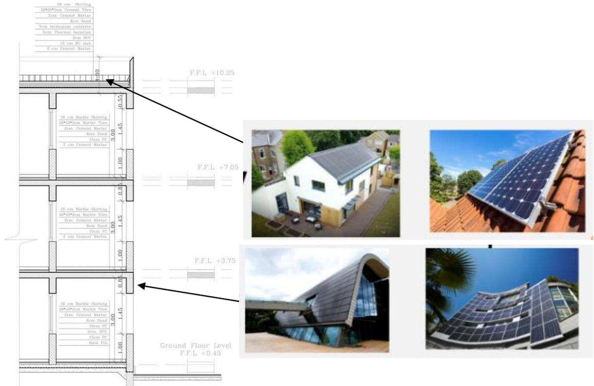
Fig. 6. Case study section with BAPV and BIPV methods (8)
