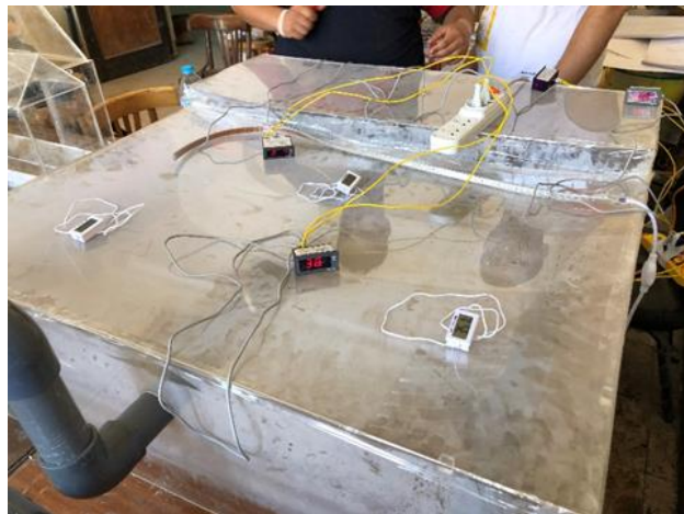
(d) Temperature sensors installed on MSJ model from outside.
