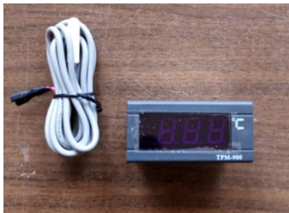
(a) Temperature sensor Ttype A accuracy 0.1 °C.
