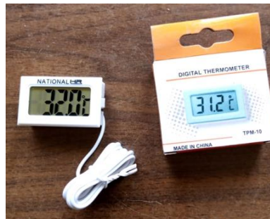
(b) Temperature sensor tType B accuracy 0.1 °C.
