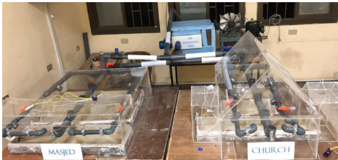
Figure 3: Experimental setup for test rig consists of two tested models MSJ-model and CHU-model, End view for test rig consists of MSJ-model (on left side), CHU-model (on right side), and AHU the back connected to refrigeration machine of air cooled condensing unit (CU).
