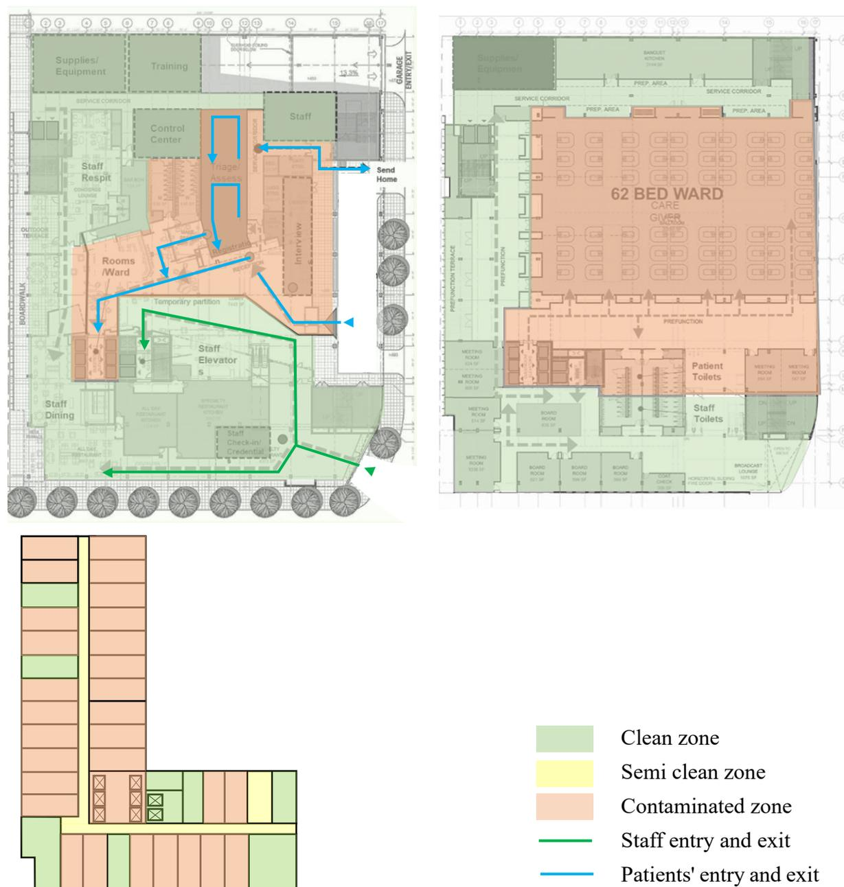
**Figure 6:** Ground, first and typical floor plan zoning by researcher based on (Schroer, Shelton, & Evans, 2020).
