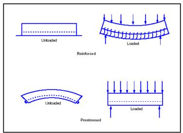
Figure (1): Difference between Reinforced & Prestressed Concrete
