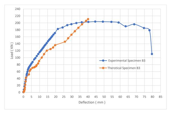
Figure (13): The Results of the Tested Beam (B3)
