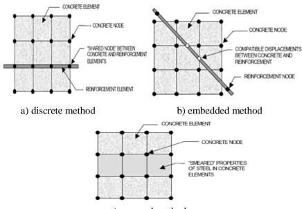
c) smeared method Figure 8: Reinforcement modeling methods (ANSYS)
