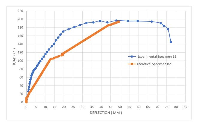
Figure 11: Comparsion between Theoretical & experimntal load-deflection curves of Tested beam
