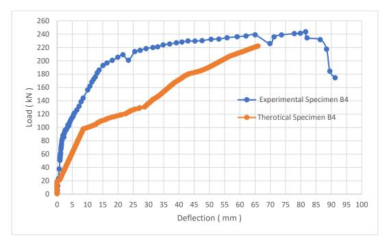
Figure (14): The Results of the Tested Beam (B4)
