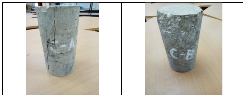
Fig. 11 Failure modes for the Two Tested Control Cylinders without CFRP Confinement, (C-A) with Cement Grade (CEM I 42.5 N) & (C-B) with Cement Grade (CEM I 52.5 N)
