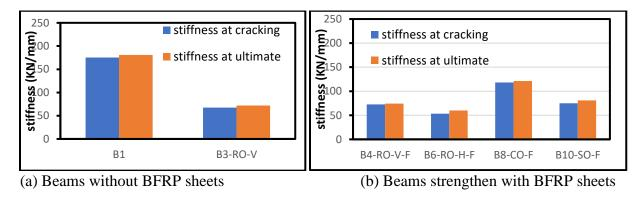
Figure (10): Stiffness at cracking and ultimate loads for all beams
