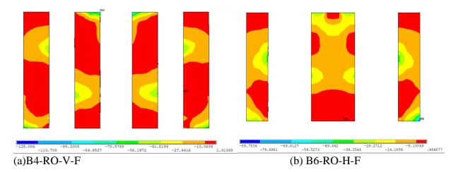
Figure (17): Normal principal stress for basalt fibbers and epoxy for some beams
