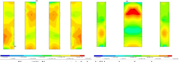
Figure (18): X-component strain for basalt fibbers and epoxy for some beams
