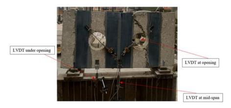
Figure (4): The locations of deflection measurement
