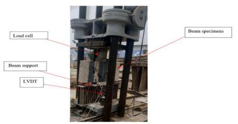
Figure (3): The test setup and loading system
