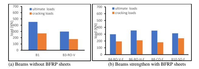
Figure (7): The first crack load and ultimate load of all beams
