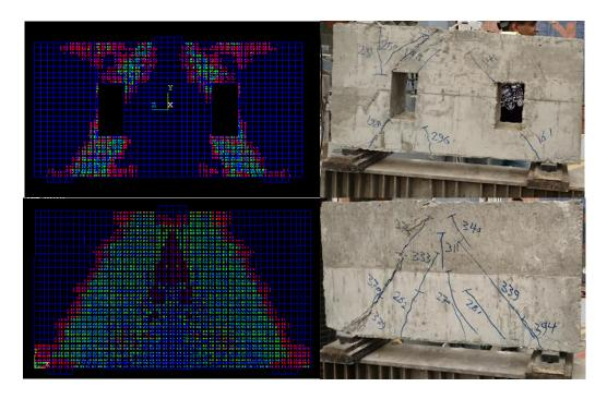
Figure (15): Comparison between nonlinear analysis and experimental crack pattern for some beams
