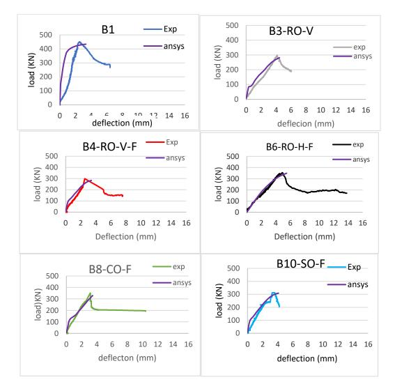
Figure (14): Comparison between ANSYS and experimental load-deflection curves for all beams
