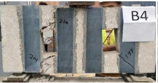
B4- RO-V-F :Diagonal-shear splitting failure failure
