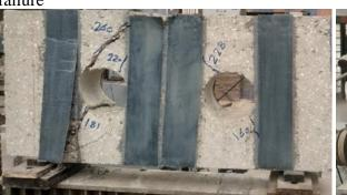
B8-CO-F: Diagonal-shear splitting failure cover splitting
