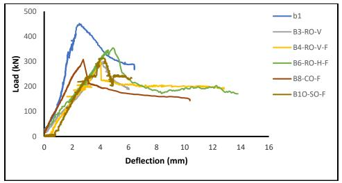
Figure (6): Load deflection curve of all beams
