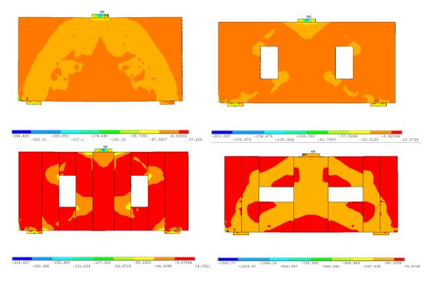
Figure (16): Normal principal stress for some beams
