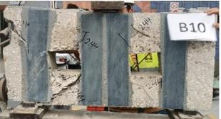
B10-SO-F: Diagonal-shear, concrete
