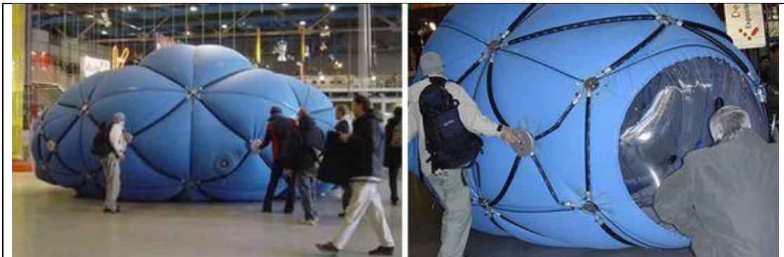
Figure 1 Kas Oosterhuis and Hyperbody Research Group. NSA Muscle. 2003. The NSA Muscle prototype has been shown at the 2003 Non-Standard Architectures exhibition at the Centre Pompidou. The structure could change its shape based on sensor orchestration of individual muscle strands due to the proximity of visitors or be steered from a more traditional screen-based interface.
