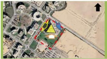
**Figure 4** the layout of the building shows the urban context of a smart village and there is no shading building in the dar alhandasa main case study, The three facades which will apply the adaptive systems (pneumatic modular system) are the North, South and Southeast facades, which are the two that have higher sunlight exposure (around 6000 [Wh] per [m<sup>2</sup>] facade in summer). **Source (Googlemaps)**
