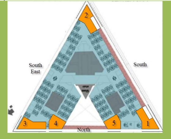
Figure 12 shows the five zones (orange colour) in the 3 directions of the building Source: adapted by the researcher
