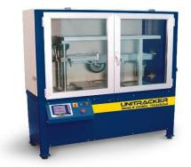
Figure (2): Rutting Test Machine
