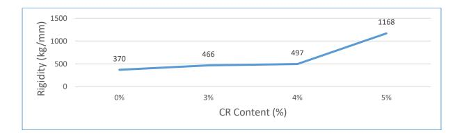
Figure (5): Rigidity for MCM with 40% RCA by weight of aggregate & Different Percentages of CR by weight of asphalt binder
