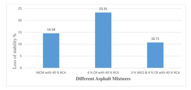
Figure (10): Shows the results of loss of stability (%) for the different mixtures
