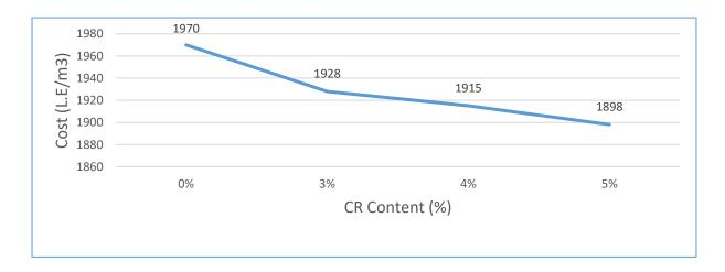
Figure (6): Cost (LE / m3) for MCM with 40% RCA & Different Percentages of CR
