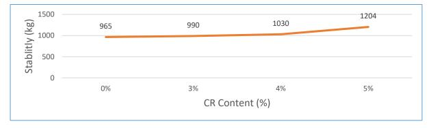
Figure (3): Stability for MCM with 40% RCA & Different percentages of CR by weight of asphalt binder
