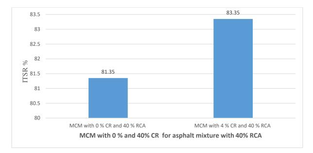
Figure (7): Percentage of Indirect Tensile Strength Ratio ITSR (%) for MCM with 40% RCA and MCM with 40% RCA & 4 % CR
