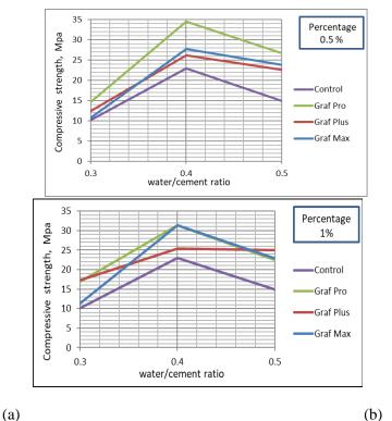
Figure 18: Comparative Compressive Strength of Tested specimens at different w/c ratios at constant nano ratio (a) at 0.5%, (b) at 1%
