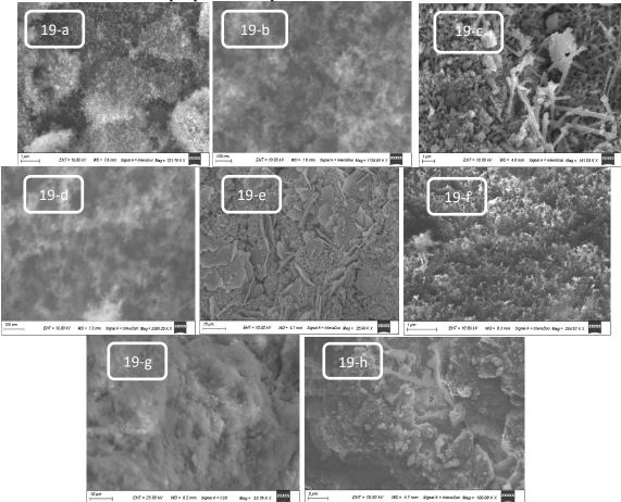
**Figure 19: SEM for tested specimens, (a:c) group G2, (d:f) group G3 and (g,h) group G4** SEM investigations of hardened mortar specimens shown that nano graphene particles are dispersed homogeneously in the mortar matrix with some agglomeration especially in samples with high proportions of nano graphene particles added (figure19-c).
