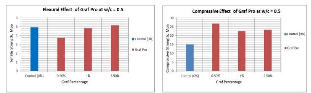
Figure 14: Flexural and Compressive Strength of Tested Specimens strengthened with Graf Pro at w/c=0.5
