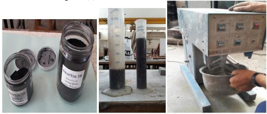
(a) (b) **Figure 1: (a) The Nano Graphene particles and (b) mixing procedure** Figure 2 shows the cement mortar specimens during casting and compacting to insure the homogeneity of cement mortar mix into the steel forum and at successive stages.
