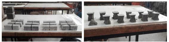
Figure 4: Failure mode of tested specimens containing different nano particles
