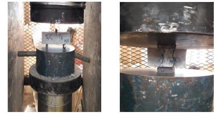
Figure 3: Test set up for flexural & compression of tested specimens According to ESS 2421-7/2005
