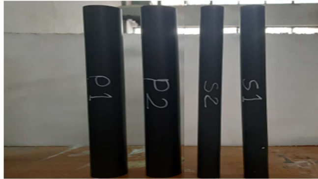
Figure 7 Round HSS samples before the test.
