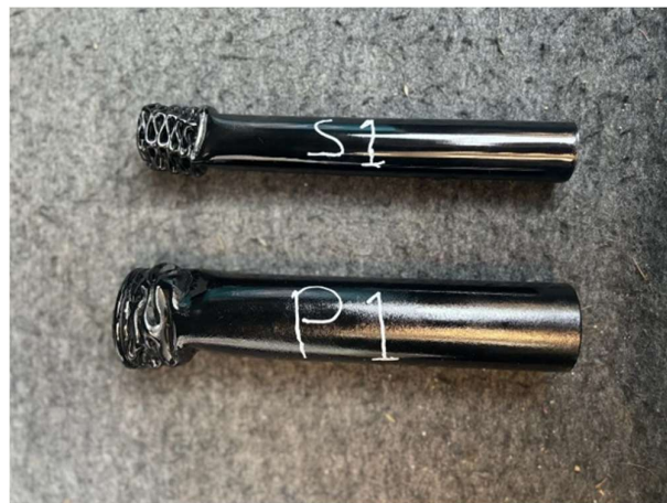
Figure 8 Axial collapse deformation behavior of two samples (P1 & S1).
