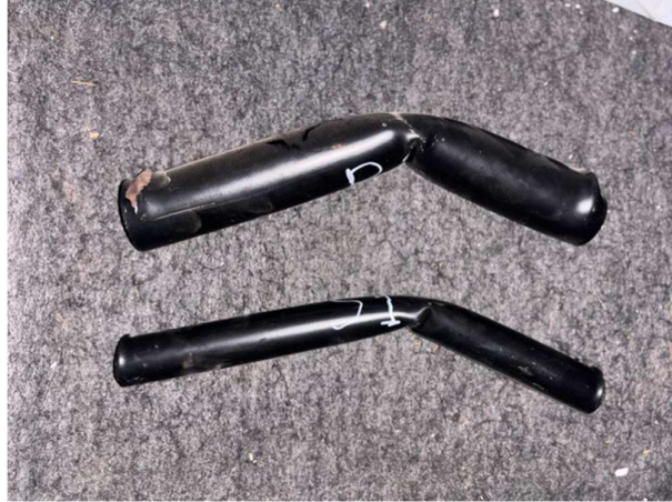
Figure 9 Bending deformation behavior of two samples (P2 & S2)
