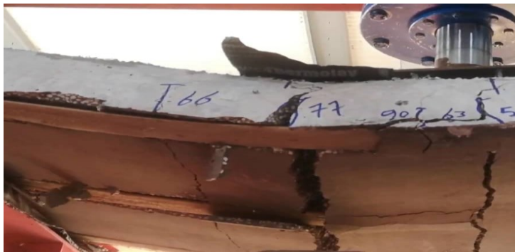
Figure 17. The crack pattern of Specimen SI350S.
