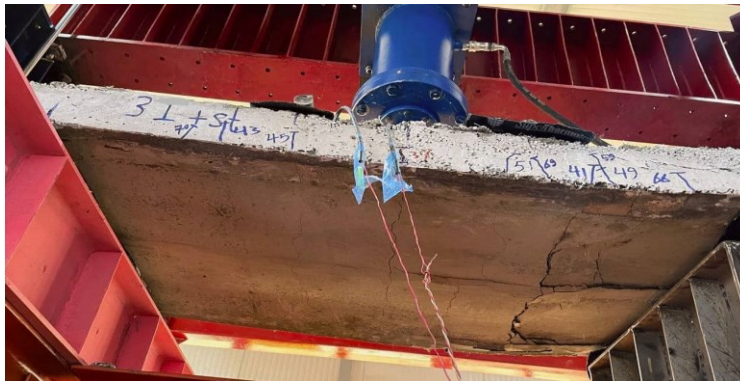
Figure 18. The Crack Pattern of Specimen ST350S.
