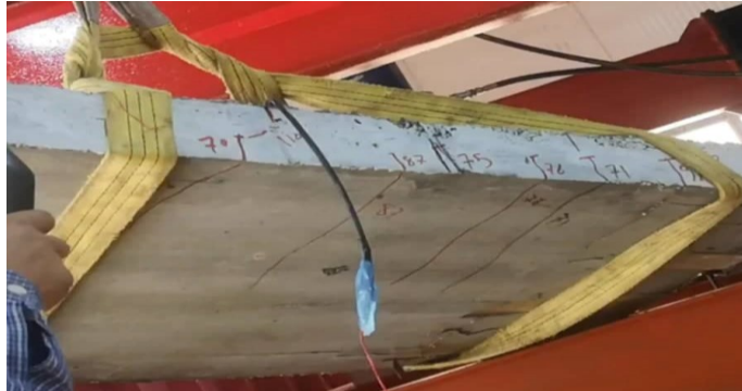
Figure 13. The crack pattern of Specimen SI233.
