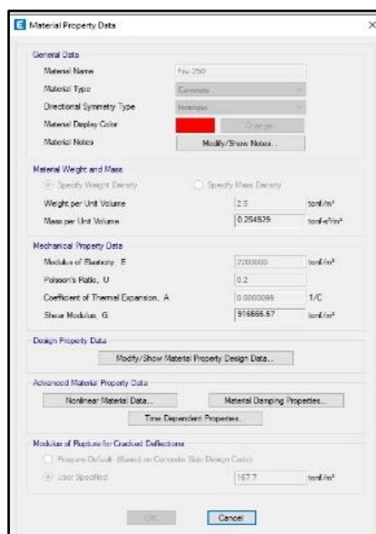
(a) Material of first model having conventional concrete for all members
