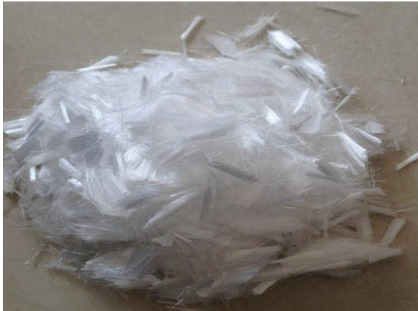
Figure 1: Incorporated polypropylene fibers (12 mm in length and 34 \mu in diameter)
