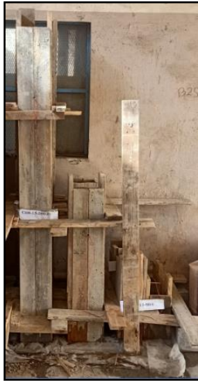
(a) Wooden forms for encased columns
