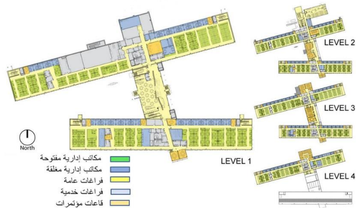
Figure 25 illustrating the horizontal sections of the administrative building to clarify the offices and common spaces.
