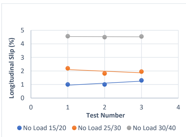
Fig.20 Longitudinal Slip Vs Inflation Pressure at No External Load
