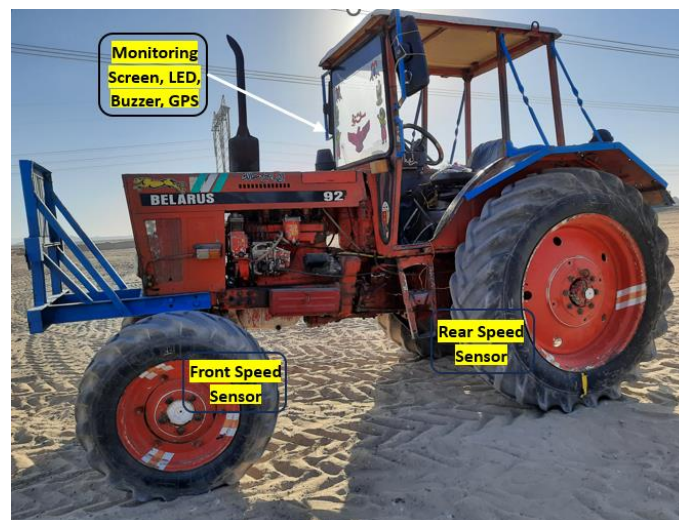
Fig. 9 Overall view of installed sensors with tractor
