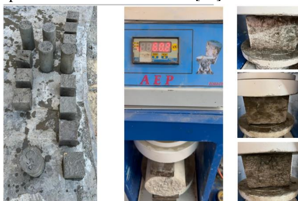
Fig. 3. Compressive strength test.
