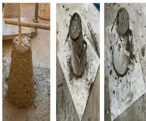
A: The slump test for the sample is 70 mm.
