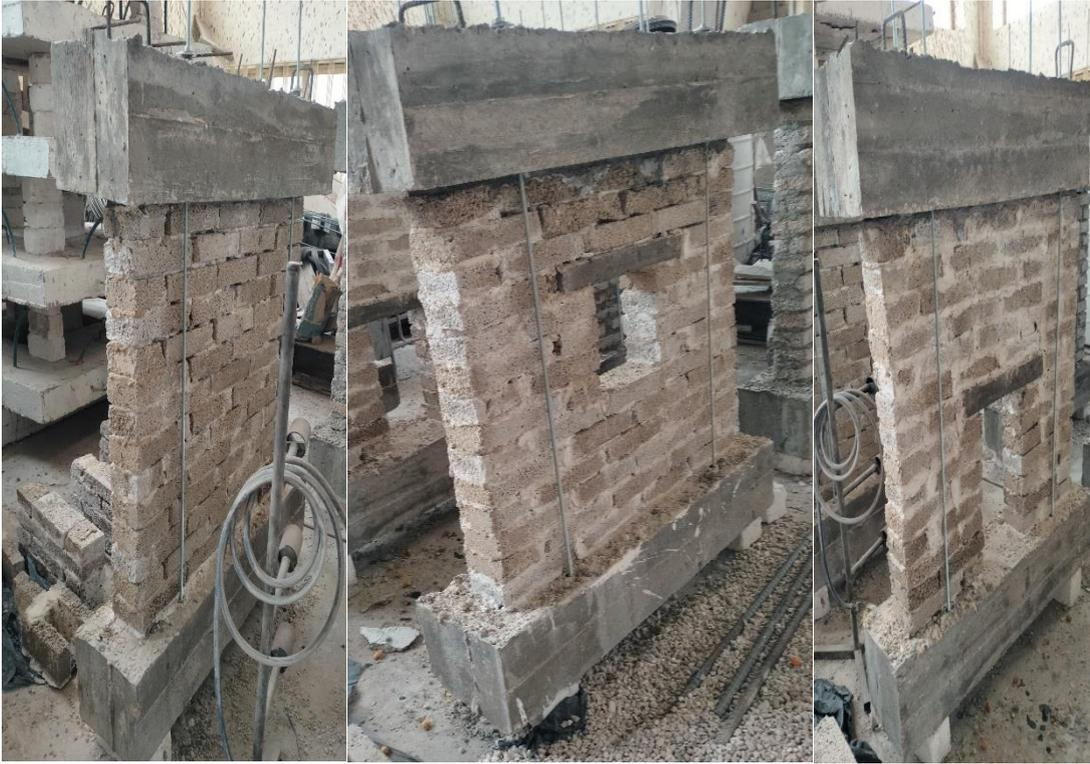
**Fig. 11:** Solid wall, window-opening wall and door opening wall made of Geopolymer brick with Geopolymer mortar.
