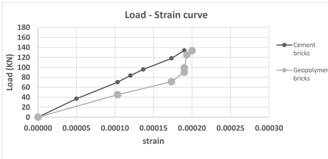
Fig. 34: Load – strain relationships for walls with door.
