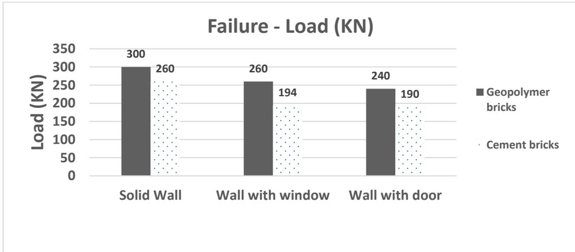
Fig. 25: Comparison of the failure load of all walls.
