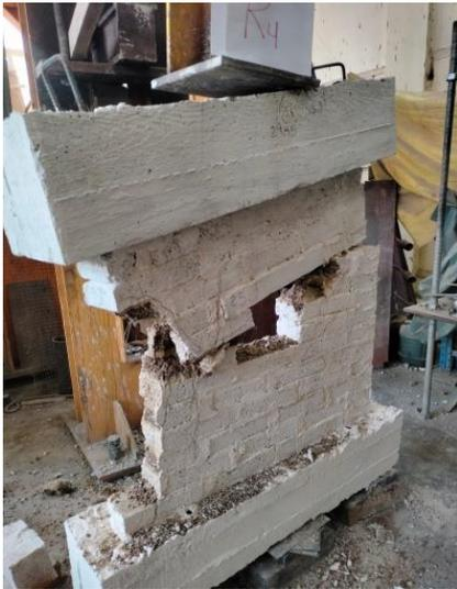
**Fig. 28:** Failure shape of Geopolymer brick wall with Window W3.
