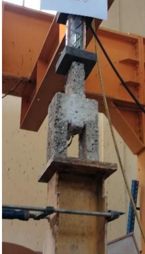
**Fig. 9:** Sample of Geopolymer prism (P7)
