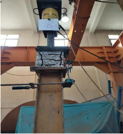
**Fig. 16:** Mode of failure of Geopolymer brick prism under load perpendicular to the bed joints (P3)
