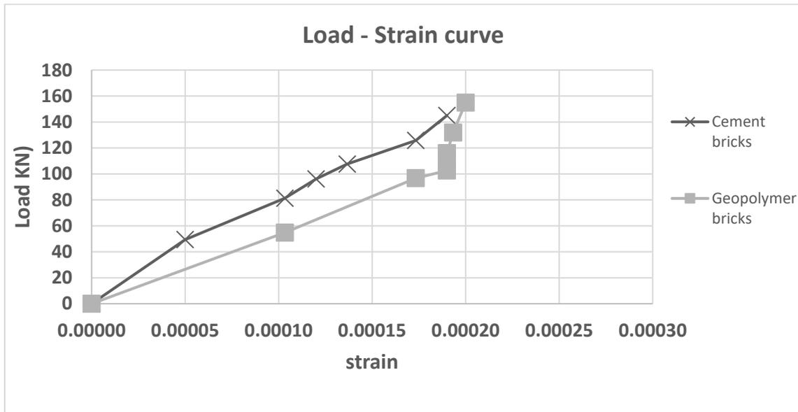
**Fig. 32:** Load – strain relationships for solid walls.
