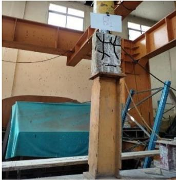
**Fig. 13:** Mode of failure of Geopolymer brick prism under load parallel to the bed joints (P1)
