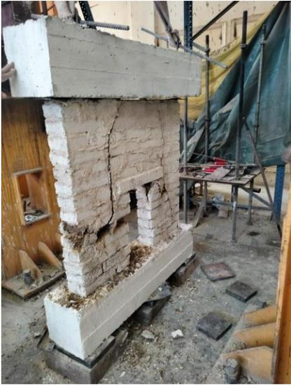
**Fig. 30:** Crack pattern and failure shape of Geopolymer brick wall with door W5.
