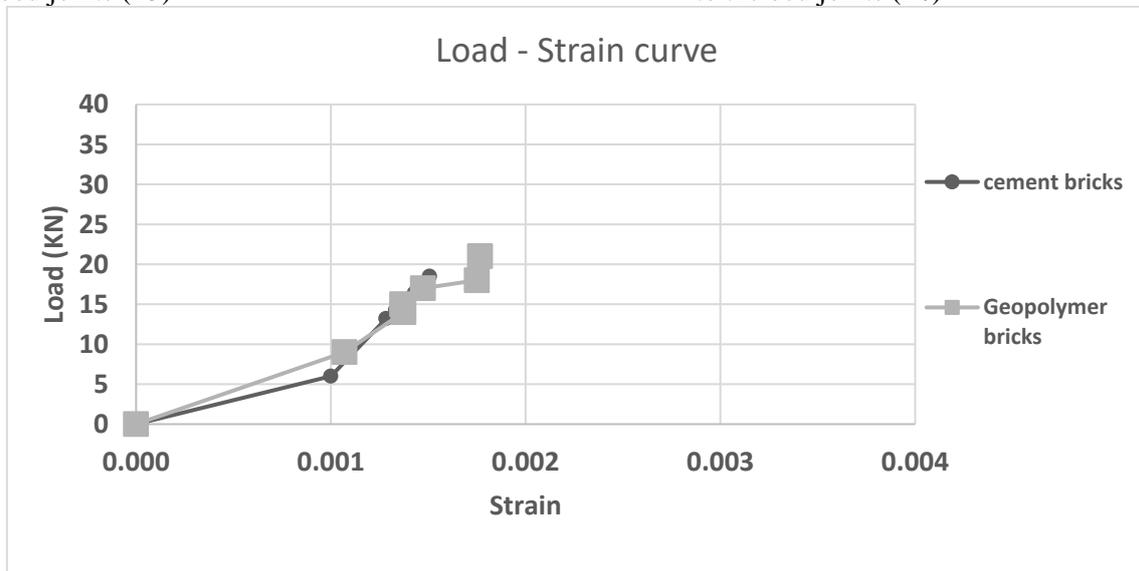
**Fig. 21:** Load -Strain relations for prisms P5 and P6 tested under vertical load perpendicular to the bed joints.
