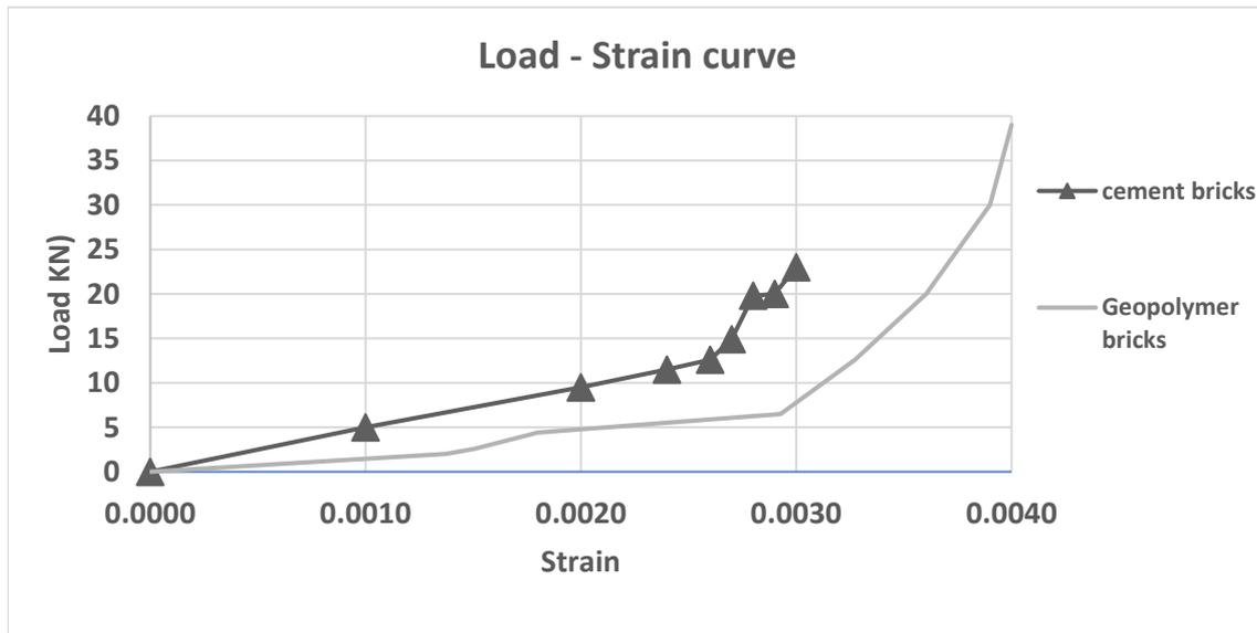
**Fig. 18:** Load-Strain relations for prisms P3 and P4 tested under vertical load perpendicular to the bed joints.
