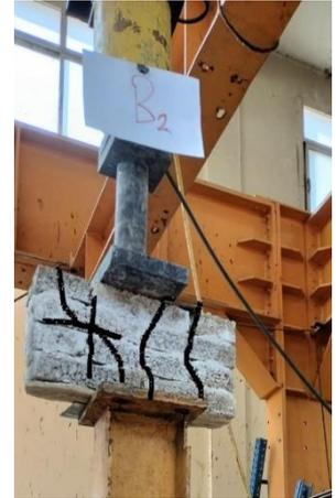
**Fig. 20:** Mode of failure of cement brick prism under load perpendicular to the bed joints (P6)
