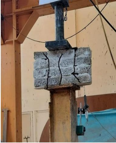
**Fig. 19:** Mode of failure of Geopolymer brick prism under load perpendicular to the bed joints (P5)
