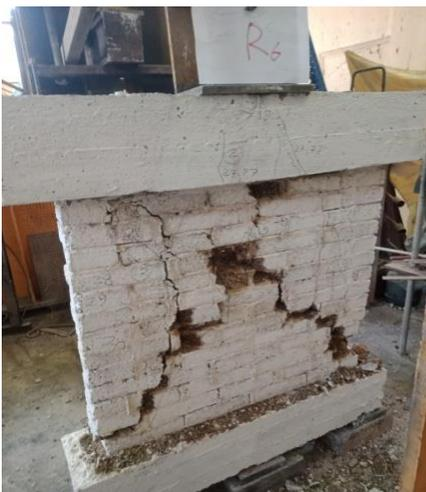
Fig. 26: Crack pattern and failure shape of Geopolymer brick solid wall W1.
