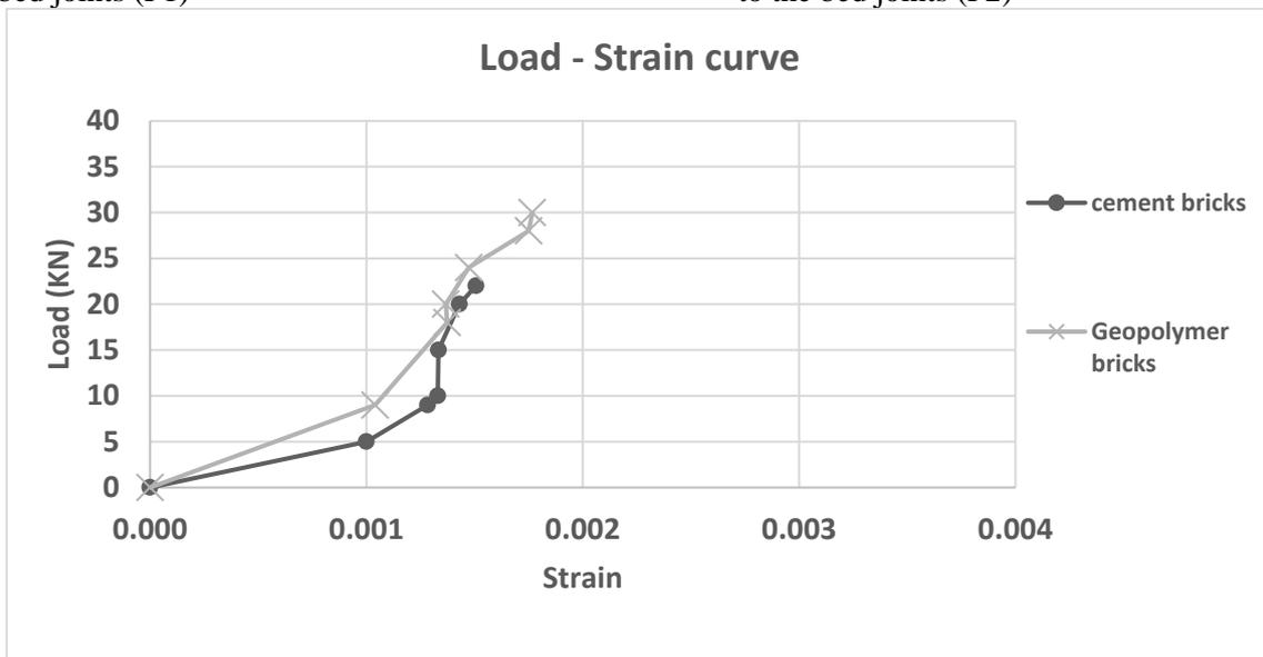
**Fig. 15:** Load –strain relations for prisms P1 and P2 tested under vertical load parallel to the bed joints.
