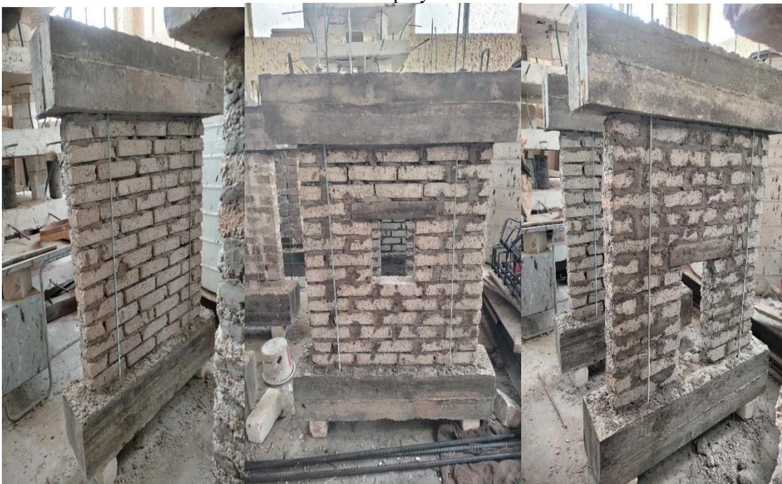
**Fig. 12:** Solid wall, window-opening wall and door opening wall made of cement brick with cement mortar.
