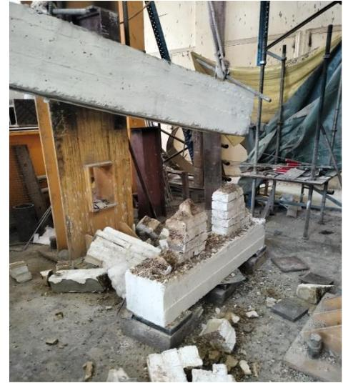
**Fig. 31:** Failure shape of cement brick wall with door W6.
