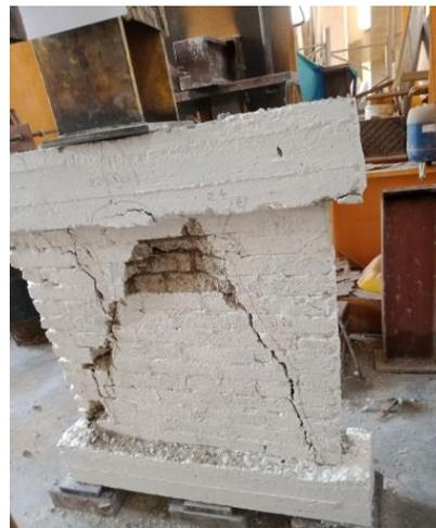
Fig. 27: Crack pattern and failure shape of cement brick solid wall W2.
