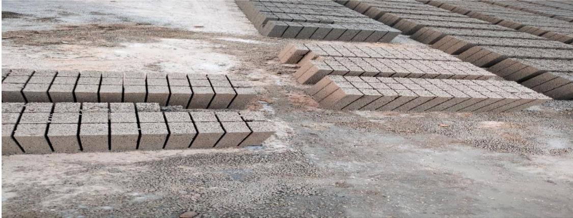
**Fig. 2:** Cement and Geopolymer bricks after casting.
