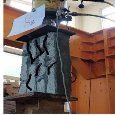
**Fig. 14:** Mode of failure of cement brick prism under load parallel to the bed joints (P2)
