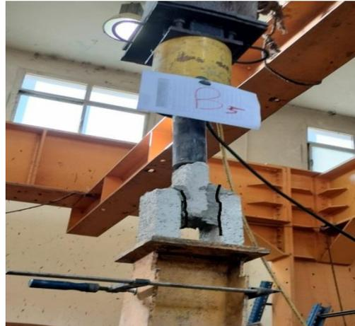
**Fig. 23:** Mode of failure of cement brick prism under load parallel to the bed joints (P8)
