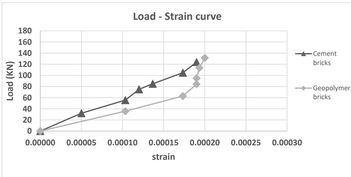
**Fig. 33:** Load – strain relationships for walls with window.
