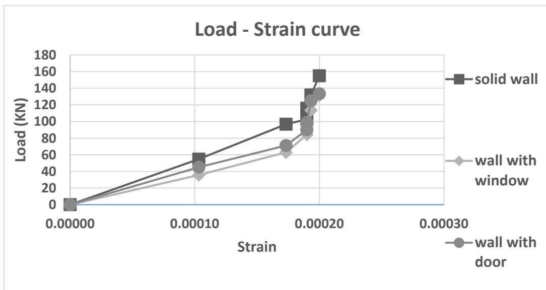
Fig. 36: Load – strain relationships for geopolymer walls.
