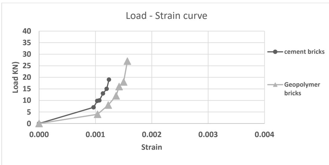
**Fig. 24:** Load –strain relations for prisms P7 and P8 tested under vertical load parallel to the bed joints.
