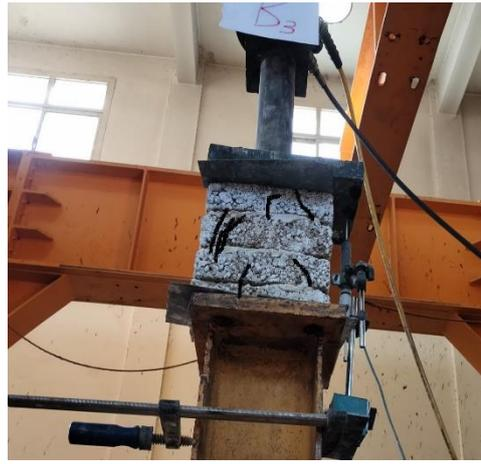
**Fig. 17:** Mode of failure of cement brick prism under load perpendicular to the bed joints(P4)
