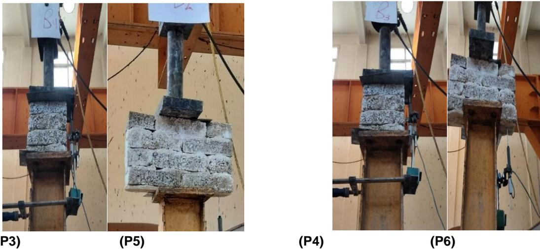
**Fig. 7:** Samples of Geopolymer prisms (P3, P5)    **Fig. 8:** Samples of cement prisms (P4, P6)
