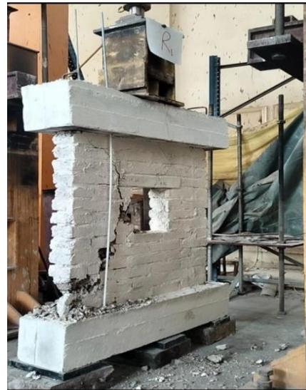
**Fig. 29:** Crack pattern and failure shape of Cement brick wall with Window W4.
