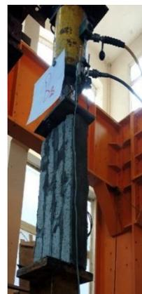
**Fig. 6:** Sample of cement prism (P2)
