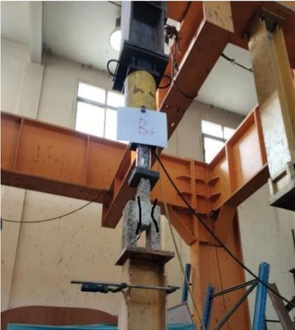
**Fig. 22:** Mode of failure of Geopolymer brick prism under load parallel to the bed joints (P7)
