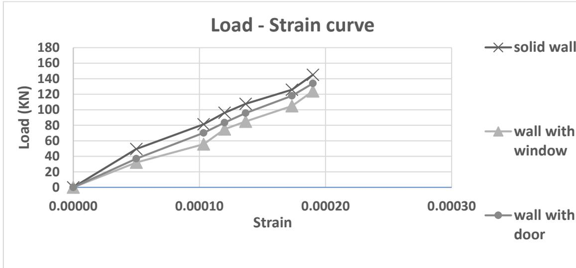
Fig. 35: Load – strain relationships for cement walls.
