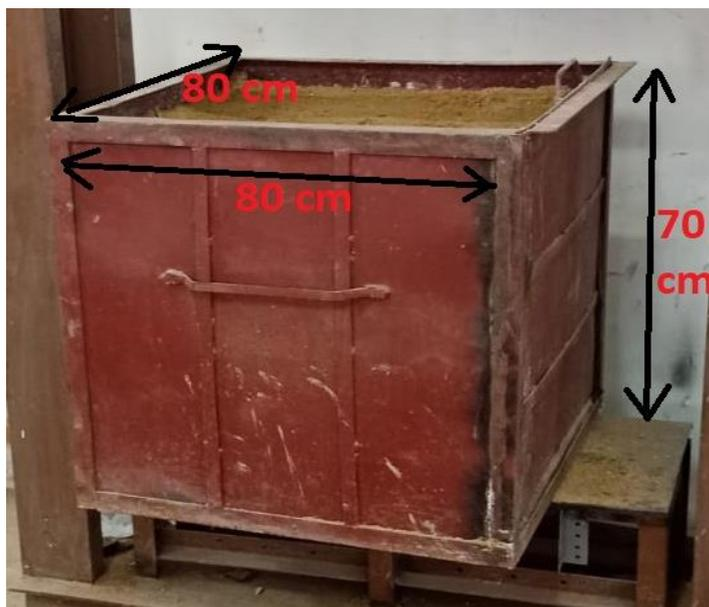
**Fig. 1.** The metal box (Container) for soil sample preparation.
