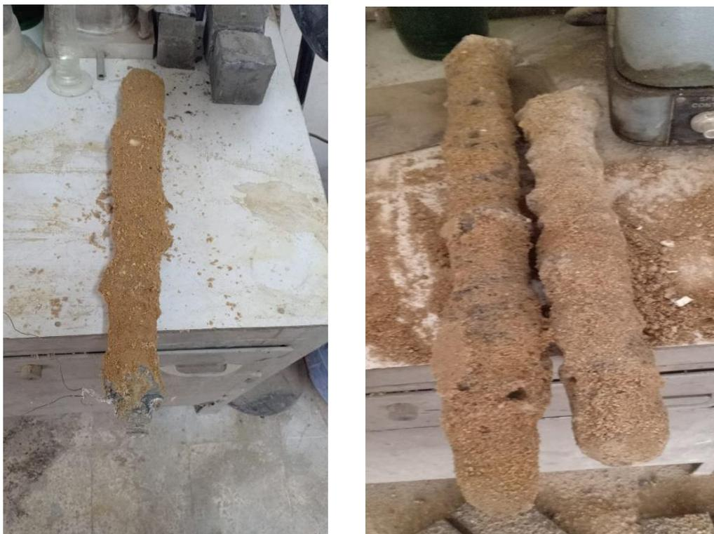
**Fig. 3.** Model micropile
