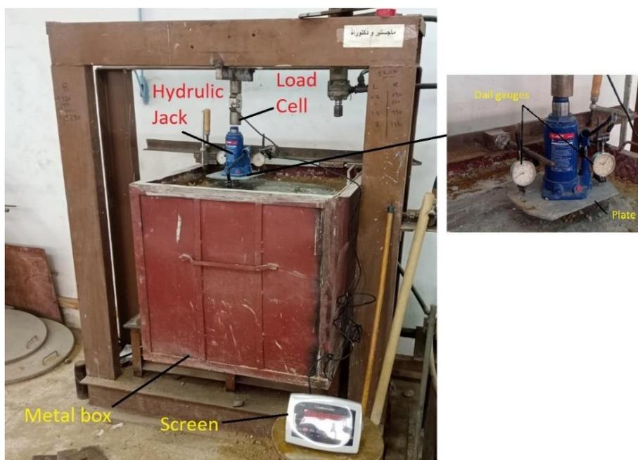
**Fig. 2.** Loading system for experimental work.
