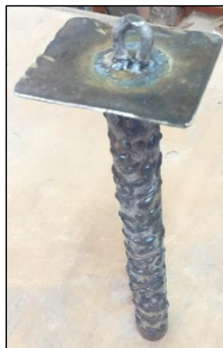
Fig.1 The model of the circular steel pile with bulges used in the present study.
