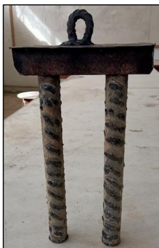
Fig. 2 The model of the (2x1) pile group.
