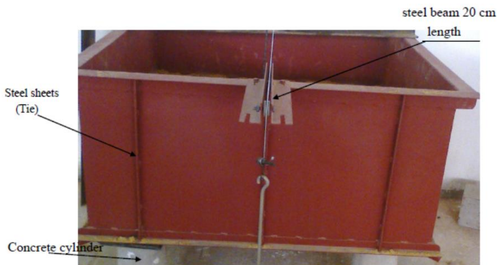
Fig. 3 The metal box (mold) for soil sample preparation.
