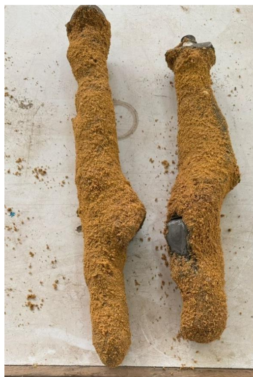
Fig. 3.b Micropile Type B after testing
