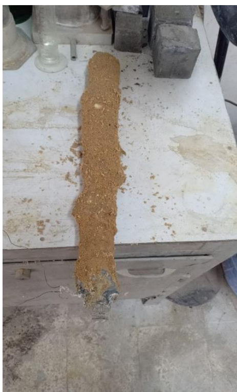
Fig. 3.a Micropile Type A after testing
