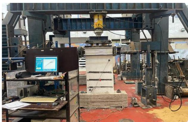
**Fig. 2:** Cyclic loading test set-up.
