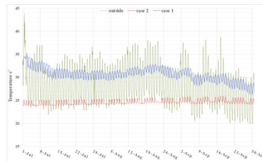
Fig. 27. Indoor temperature data analyzed in summer (with and without PCM)
