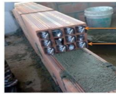
Fig. 17. Integration of PCM in hollow brick. [40]
